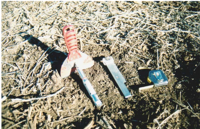
Figure 3. The Modified Singleton Blade and the original blade at the site for the data are in Tables 1 and 2. The measuring tape is extended to 5 cm.
