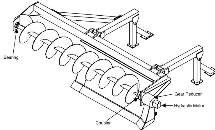
Figure 3. Illustration of support structure, helicoid auger, and drive components.
