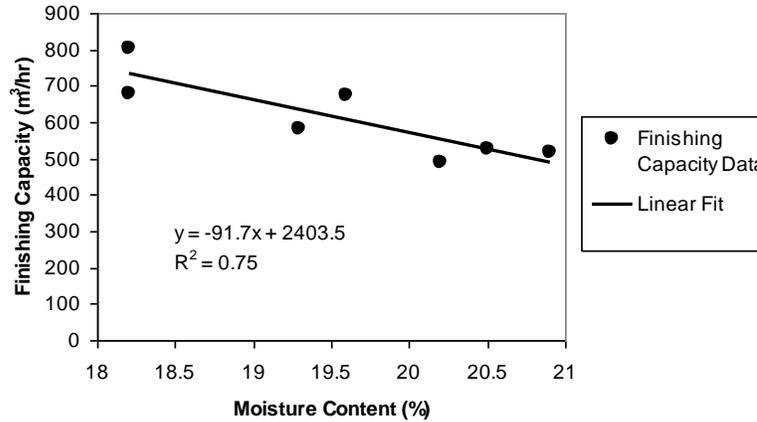
Figure 11. Finishing capacity versus moisture content.
