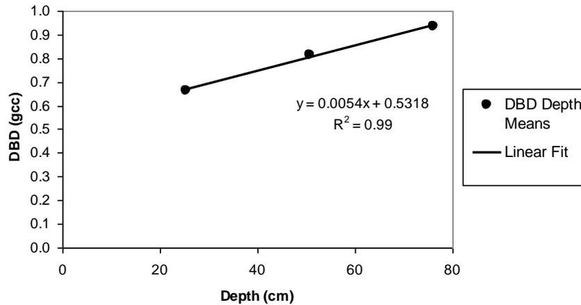
Figure 13. Mean DBD versus depth for all three berms.
