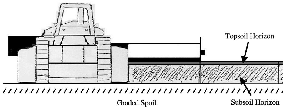
Figure 5. Soil placement from successive parallel passes.
