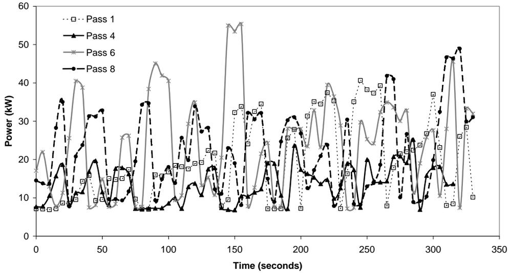
Figure 9. Auger power versus reconstruction time collected for several passes.
