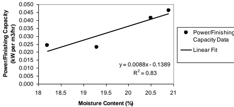
Figure 12. Power/finishing capacity versus moisture content.
