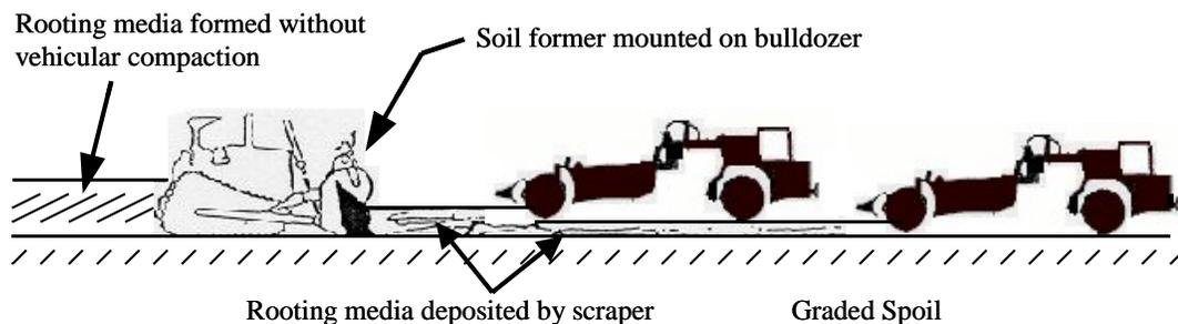
Figure 4. Soil handling process with mechanism loosening and reconstructing soil deposited in a windrow.
