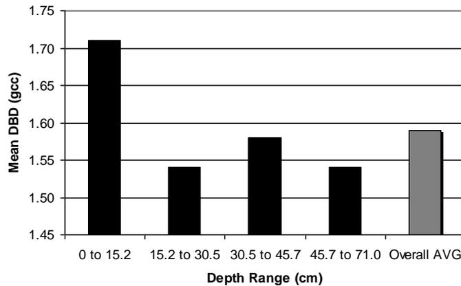
Figure 14. Mean DBD for all four-depth ranges plus overall average for conventionally reconstructed soil at the Grand Eagle mine.
