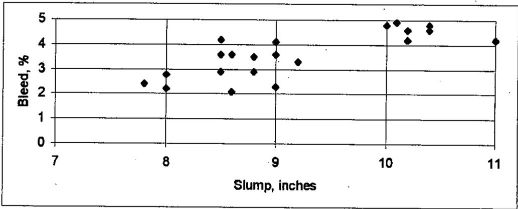
Figure 8 Relationship between slump and bleed
