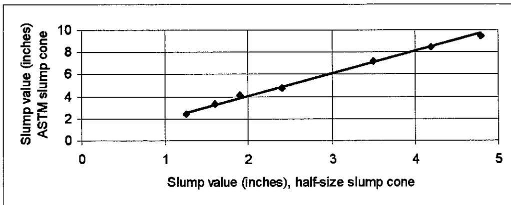
Figure 1 Relationship between ASTM slump and half-size slump
