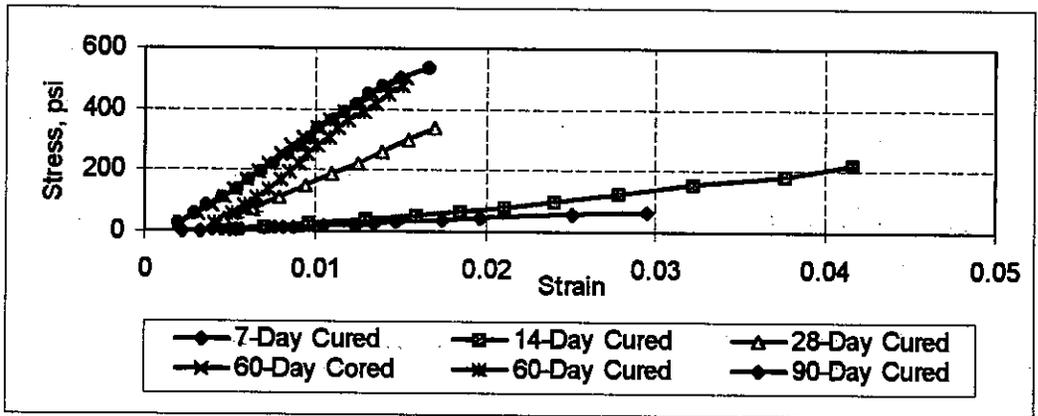
Figure 9 Typical stress-strain profiles of samples
