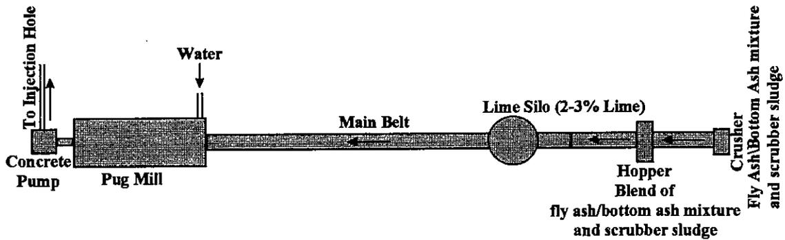
Figure 2 Schematic of mixing plant for hydraulic placement
