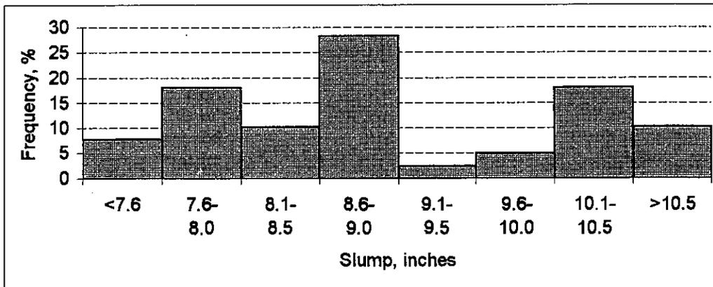
Figure 6 Frequency distribution of slump measurements
