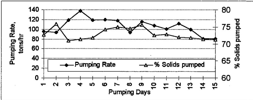
Figure 4 Pumping rate and percentage solids pumped
