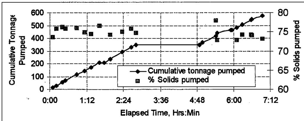
Figure 5 Percentage solids pumped in a typical pumping day
