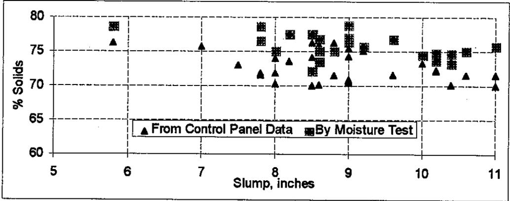
Figure 7 Slump vs. % solids of grouts
