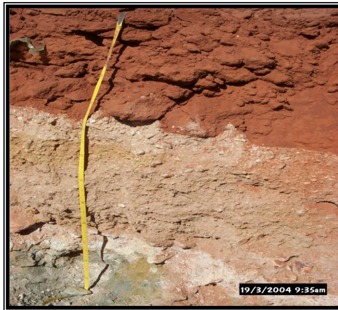
Plate 7 Capping material over acid waste material
