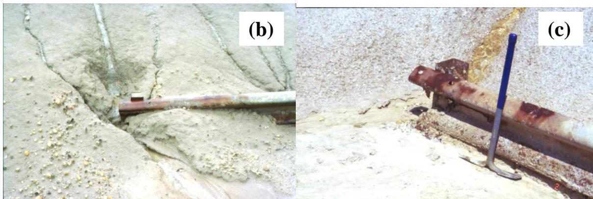
Figure 2. (a) This road cut along the cloverleaf of Rt-360W to I-295S, near Mechanicsville, Virginia, exposes the Eastover and Calvert formations of the Chesapeake Group. Sulfide oxidation has created extremely acid surface soil conditions ( $\text{pH} < 3.5$ ). (b) A few years after construction, erosion began to expose the end of this metal guardrail further, and corrosion is evident. (c) Within 5 years, erosion has removed over 30 cm of sediment and the metal is severely corroded.
