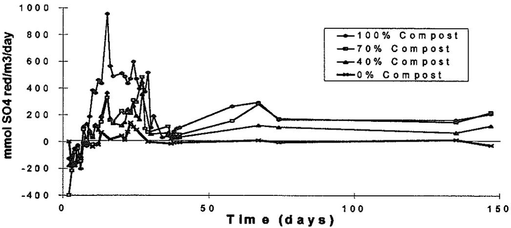
Figure 5. Sulfate removal rate was plotted over time. Significant sulfate reduction was observed in all columns with organic content.
