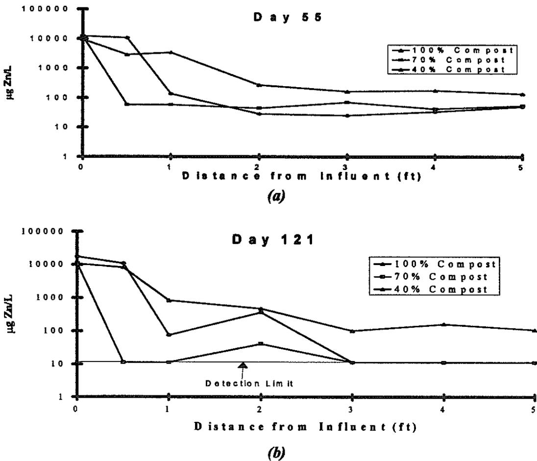
Figure 6. Zinc concentrations over the lengths of the columns at day 55 (a), and day 121 (b). Zinc was removed faster in the columns with higher organic compost fractions.
