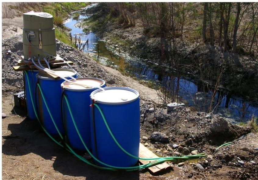
Figure 1. Bioreactors at field test site.
