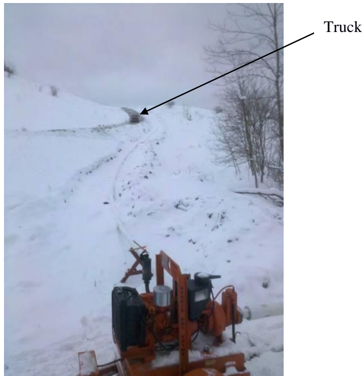
Figure 2. One of two CD103M pumps used for Test 1. A pickup truck located in the background provides scale.
