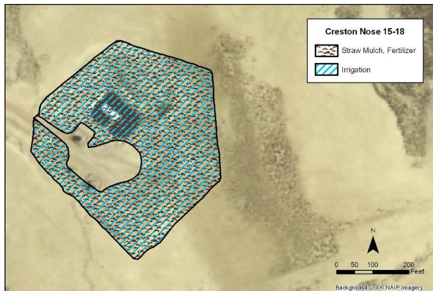
Figure 11. Illustration of reclamation treatments implemented on a 1.73 ha area located at Creston Nose 15-18.
