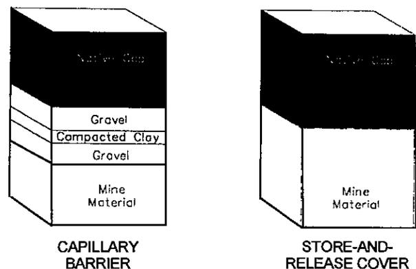
Figure 9. Capillary barriers and store-and-release cover designs
