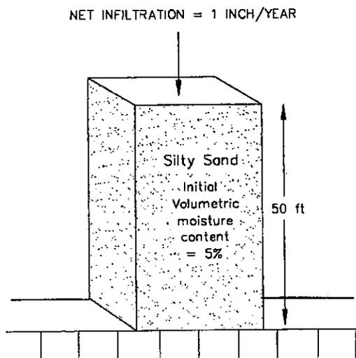
Figure 10. Example profile of sand to illustrate wetting
