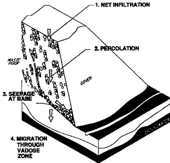
Figure 1. Hydrologic components of a waste rock facility
