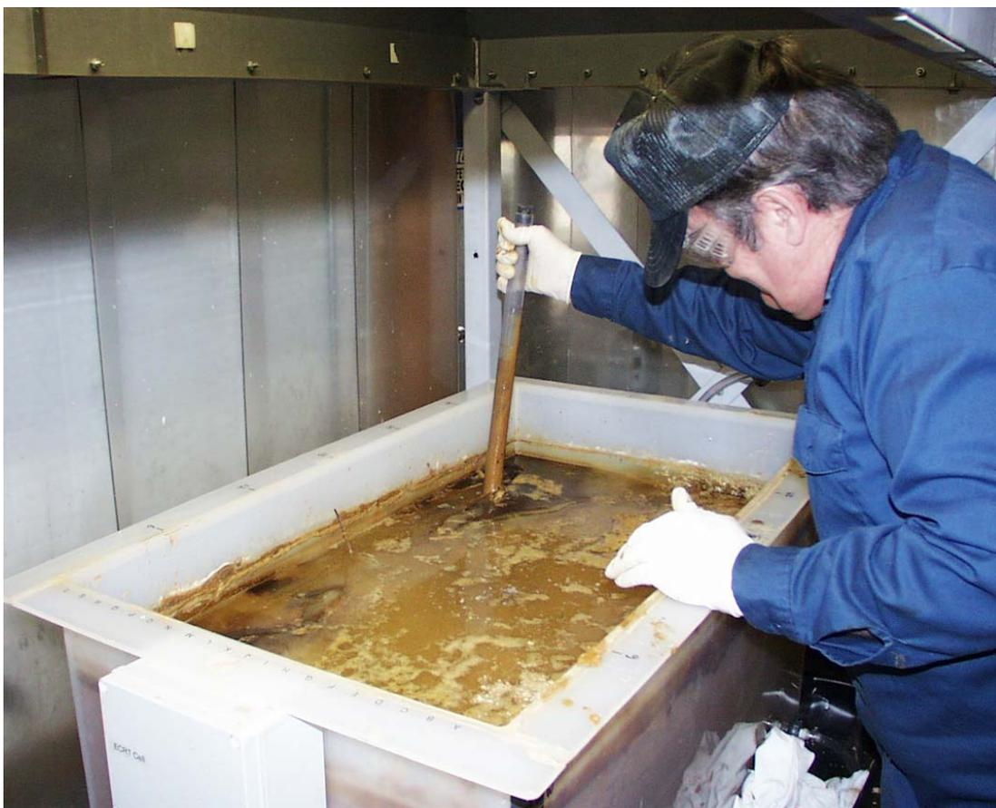
Figure 7. Test array and sampling during ECRTs tank-scale testing of soil from U.S. Department of Energy Oak Ridge Y-12 plant.
