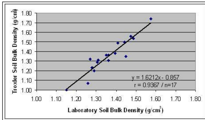
Figure 4. Linear regression between the Troxler gauge and laboratory determined dry soil bulk density (n=17).
