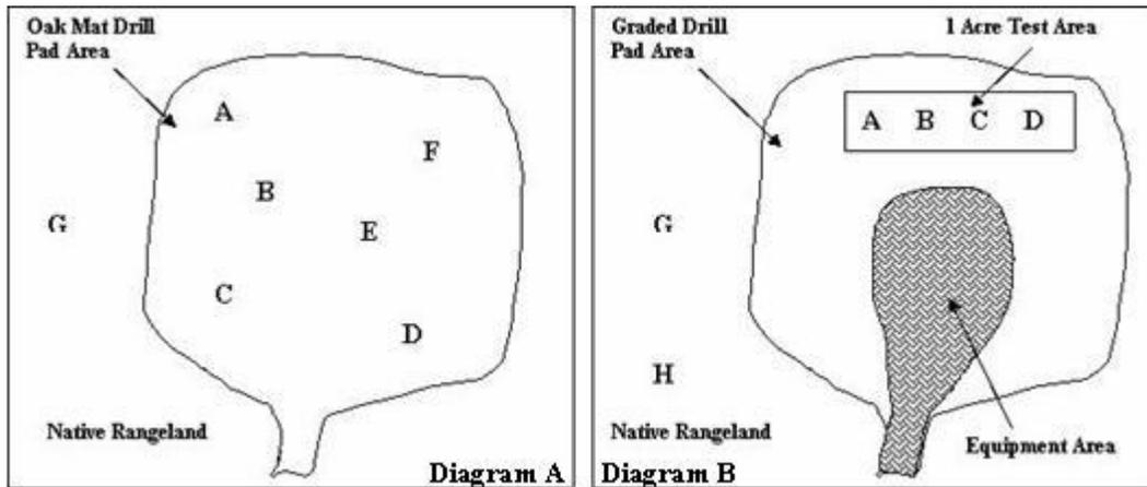
Figure 3: Plan view of generalized bulk density measurement locations at oak mat (diagram A) and conventional drill pad locations (diagram B).
