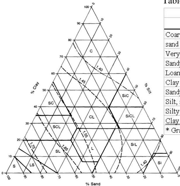
Figure 5. Isodensity lines ( $\text{g/cm}^3$ ) based on soil texture that represent growth limiting bulk densities.
