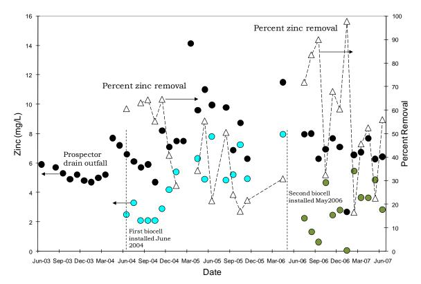
Figure 5. Pilot Scale Results. Solid circles are influent (Prospector outfall) Zn concentration (left axis), circles filled with blue are effluent concentration from first pilot scale
