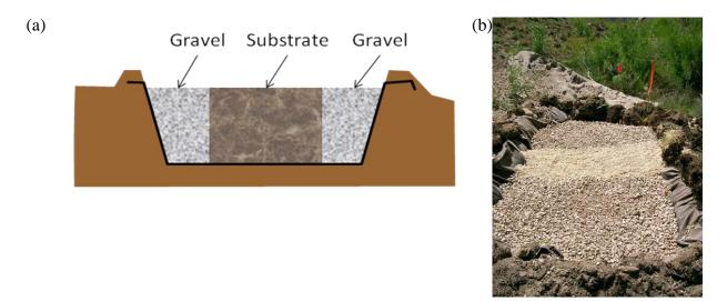
Figure 2. (a) Section showing first pilot unit design. (b) image of construction.
