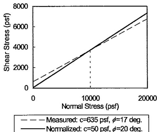
Figure 1. Normalization of measured shear strength parameters by rotating failure envelope.
