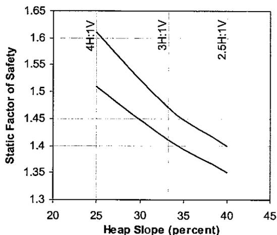
Figure 5. Upper and Lower Bounds for the static Factor of Safety for which the Pseudo-static Factor of Safety Equals One for a seismic coefficient of 0.1.
