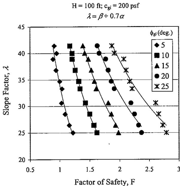
Figure 2. Example results of stability analyses showing power type curve fit to data points.
