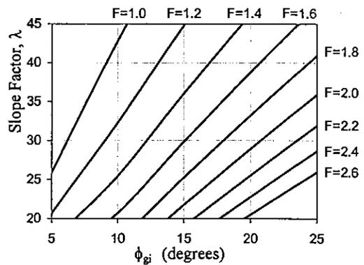
Figure 3. Stability Charts for the Case of the Ore Sliding on the Leach Pad Liner, Obtained Using Spencer's Method of Slices.
