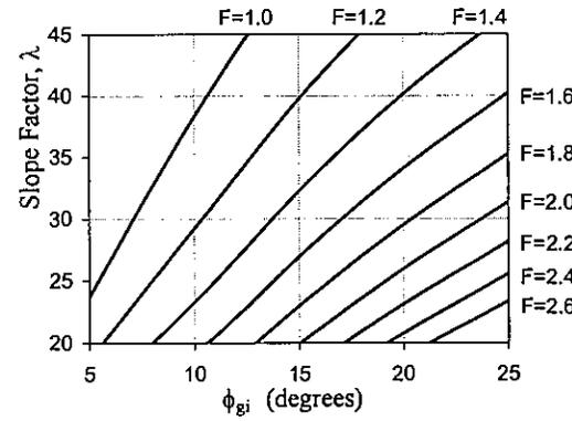
Figure 4. Stability Charts for the Case of the Ore Sliding on the Leach Pad Liner, Obtained Using the Simplified Janbu Method of Slices.
