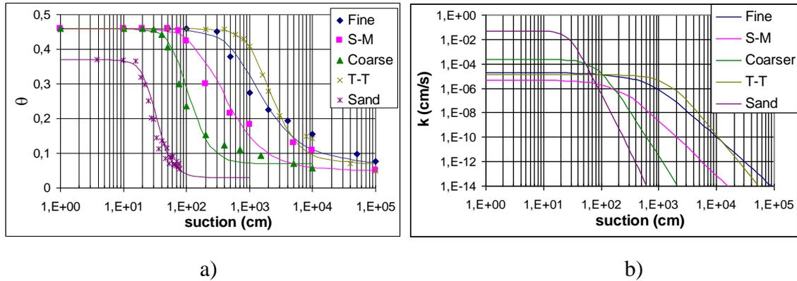
Figure 3. Hydraulic functions used in the numerical study a) WRC b) k functions; based on the Mualem (1976)-van Genuchten (1980) model.
