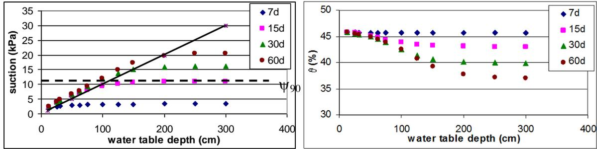
Figure 4. Calculated values of  $\psi$  (a) and  $\theta$  (b) for a point located 2 cm below the S-M tailings surface, as a function of the depth of the water table, for different drainage period.
