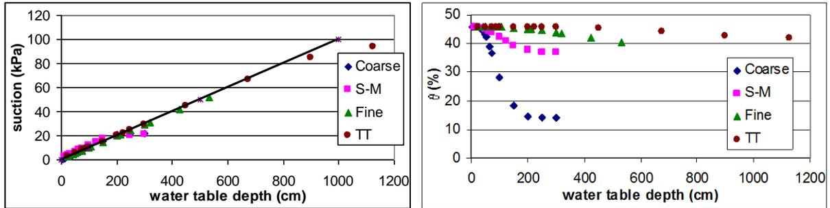
Figure 5. Calculated values of  $\psi$  and  $\theta$ , for a point taken at 2 cm below the surface of the four tailings, as a function of the depth of the water table, after 60 days of drainage.
