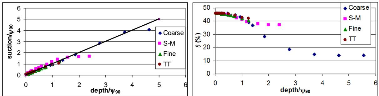
Figure 6. Normalized  $\psi$  and  $\theta$  calculated at depth of 2 cm below surface of the four tailings, as a function of the normalized water table depth, after 60 days of drainage.
