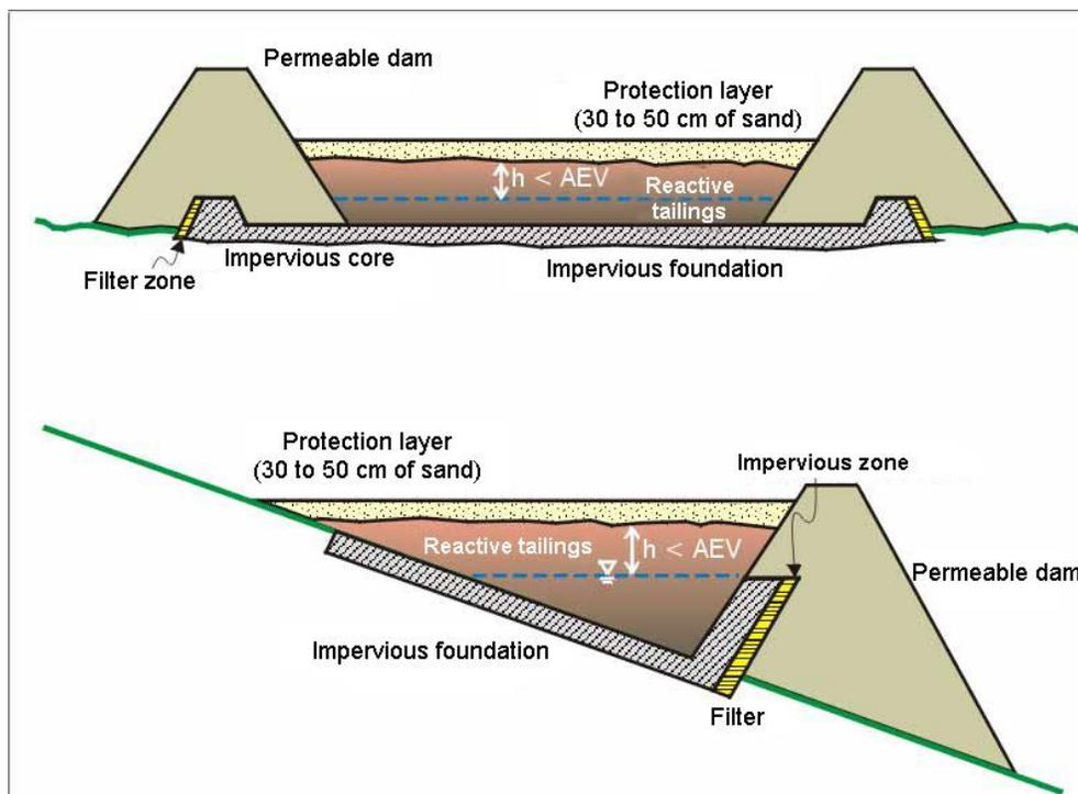
Figure 2. Conceptual view of a tailings impoundment with the phreatic surface positioned to maintain an “elevated water table” (Aubertin et al., 1999).
