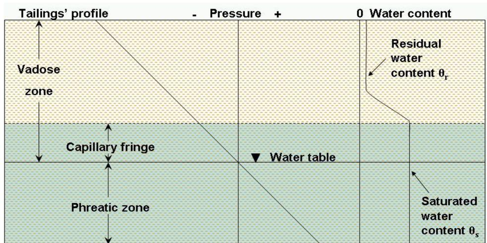
Figure 1. Conceptual view of a tailings profile showing pressure and water distribution (adapted from MEND, 1996).
