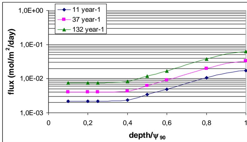
Figure 7. Oxygen flux calculated, as a function of the normalized depth, for different  $K_r$  after 30 days of drainage.
