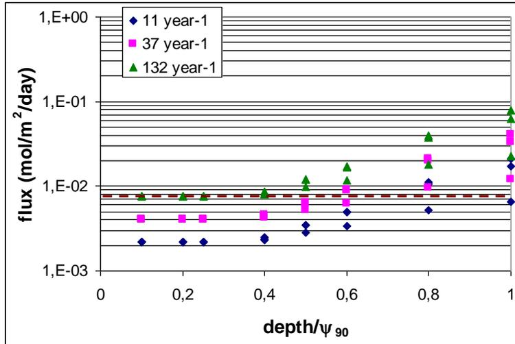
Figure 8. Calculated values of the O<sub>2</sub> flux, as a function of the normalized depth, for different K<sub>r</sub> values and drainage period.
