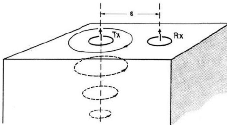
Figure 2. Induced current flow, where Rx is the receiver coil, Tx is the transmitter coil, and s is the intercoil spacing. Figure from McNeill, 1980b page 5.
