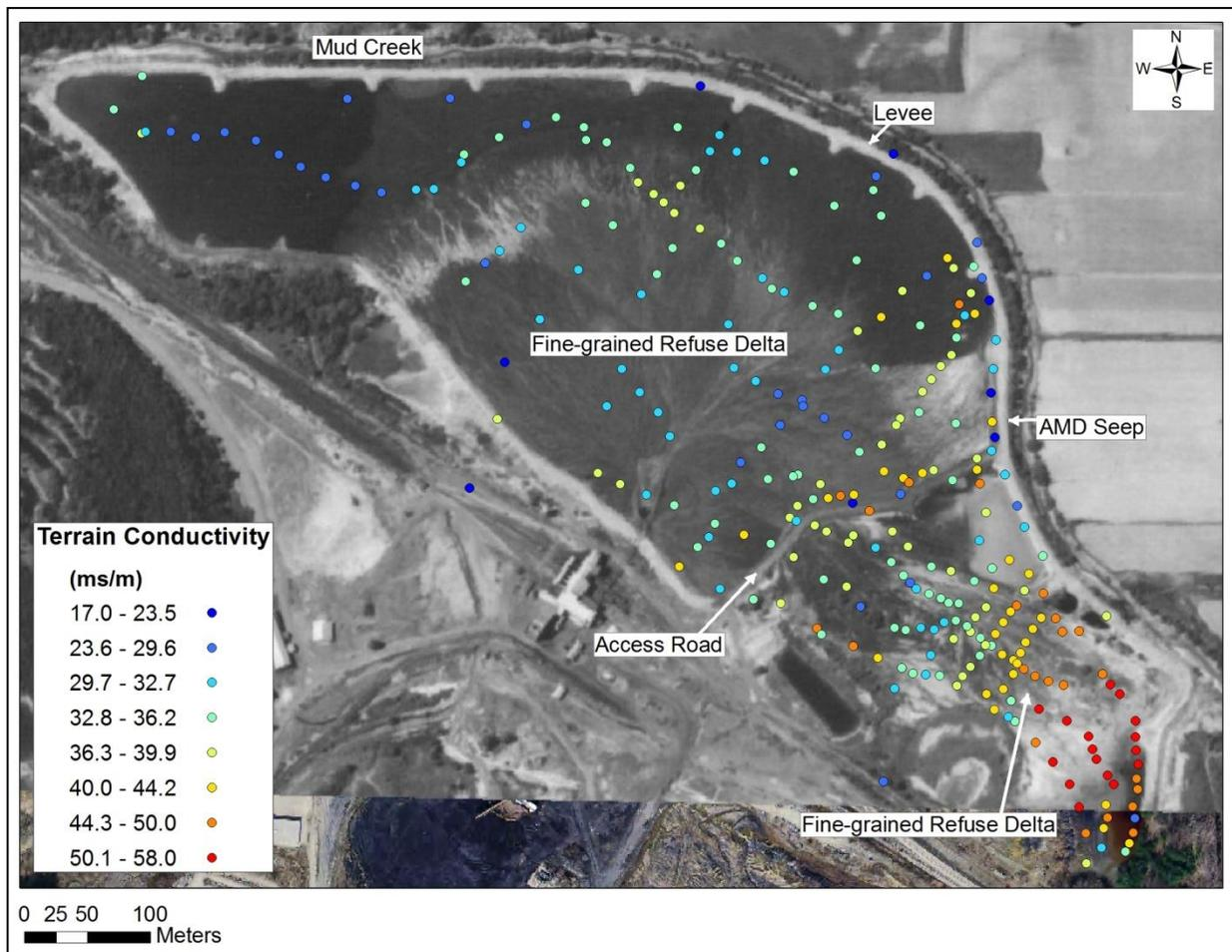
Figure 3. Terrain conductivity measurements plotted over a 1954 aerial photo of active refuse deposits.
