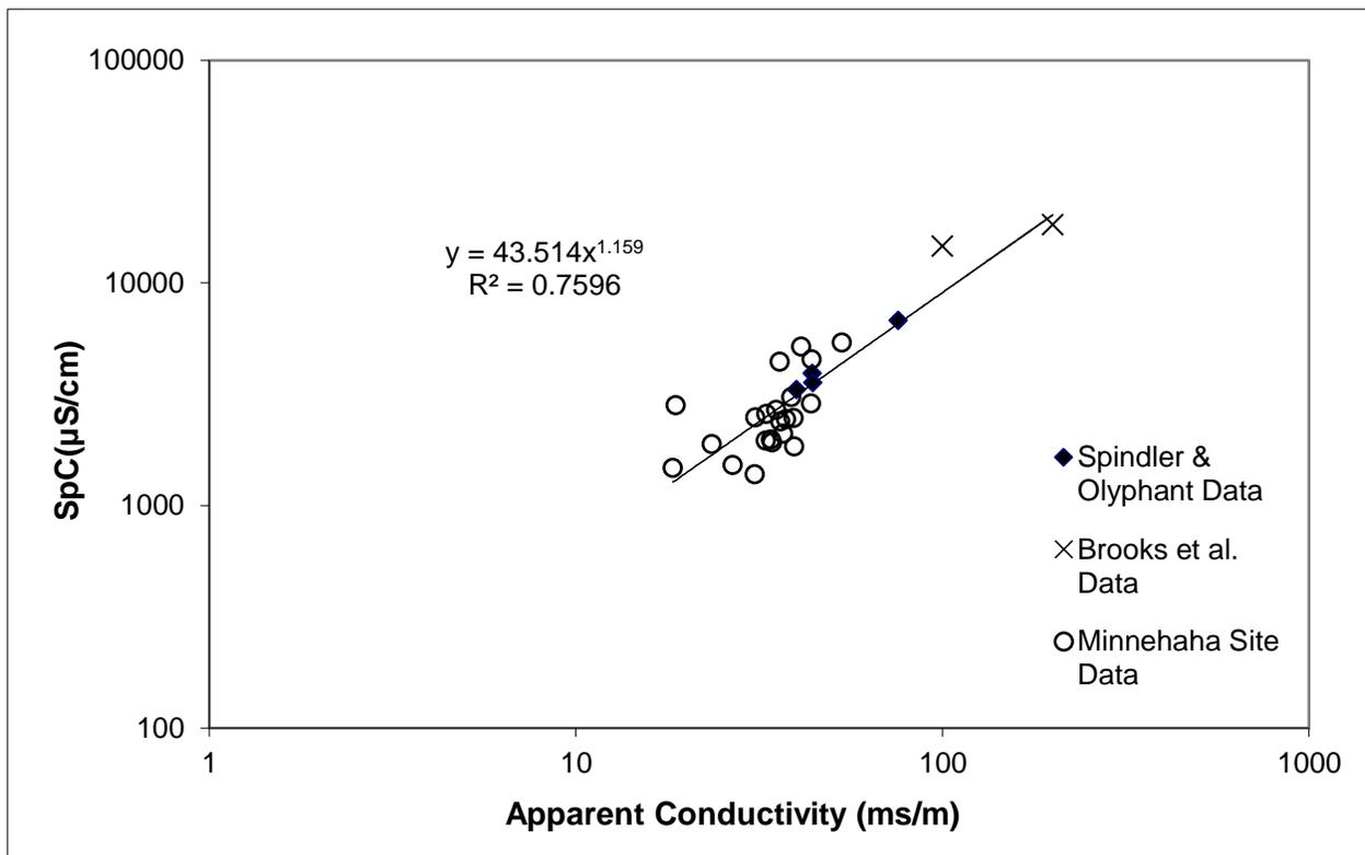
Figure 5. Plot showing relationship between apparent conductivity (terrain conductivity) and porewater SpC for three AMD sites in southwestern Indiana (Figure 1).
