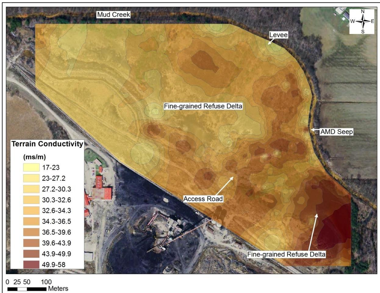
Figure 4. Aerial photo of Minnehaha abandoned mine land with interpolated terrain conductivity measurements. An inverse distance weighting method was used for interpolation.
