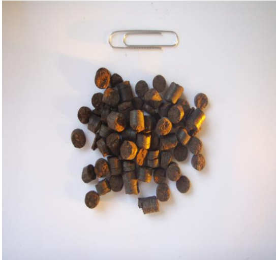
Figure 5. Peat pellets ion exchange media
