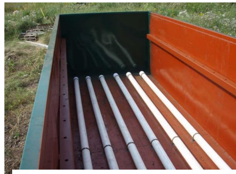
Figure 8. Drainage collection system
