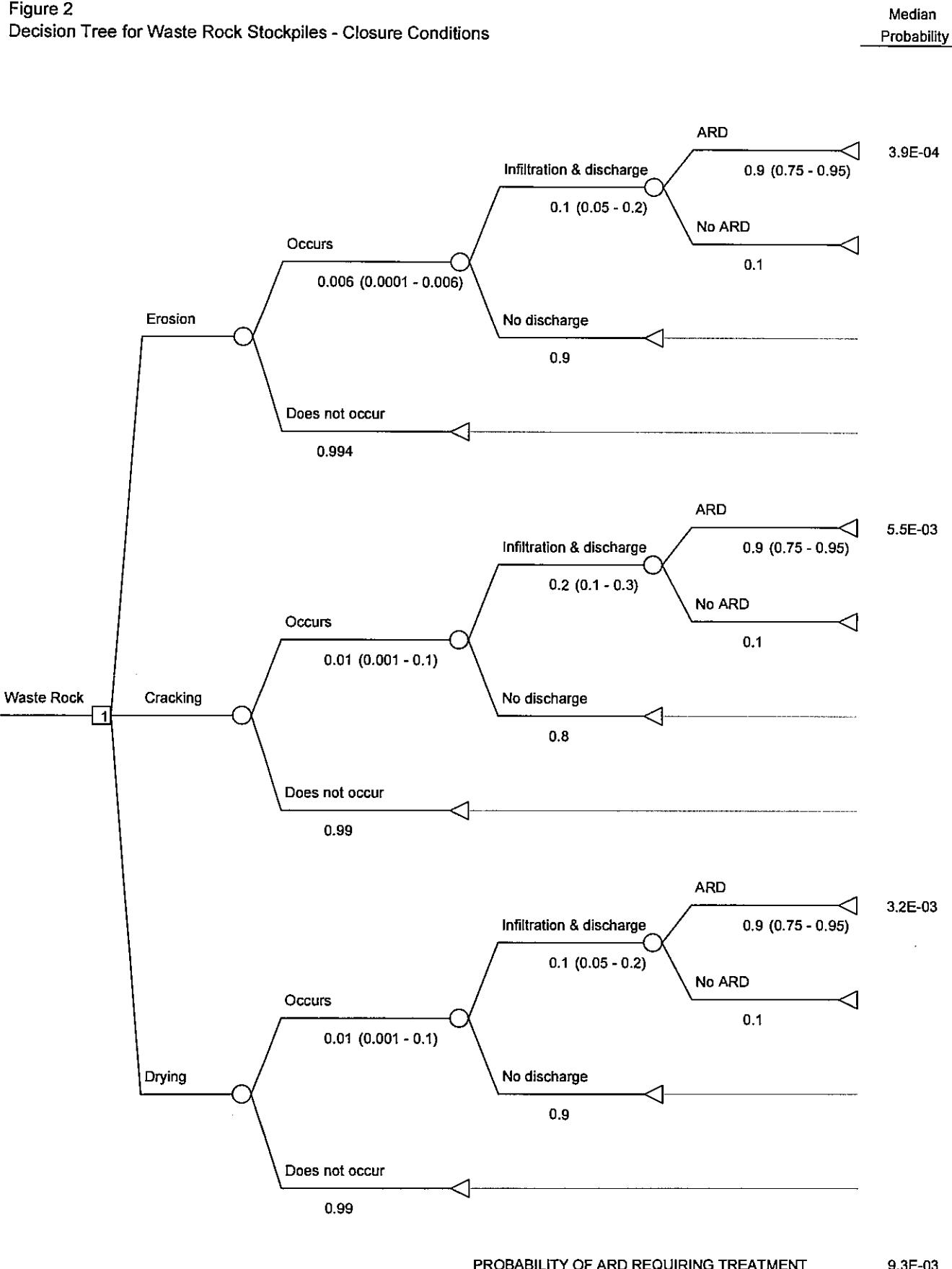
Under the maximum expected sheet erosion rate of 3.5 mm/year, it would take 171 years for the PCL to be compromised, assuming a cover thickness of 600 mm of topsoil over the PCL. Therefore, placement of the cover section proposed in the Rehabilitation and Closure Plan significantly reduces the probability of waste rock erosion from current conditions, when the cover section is incomplete.
