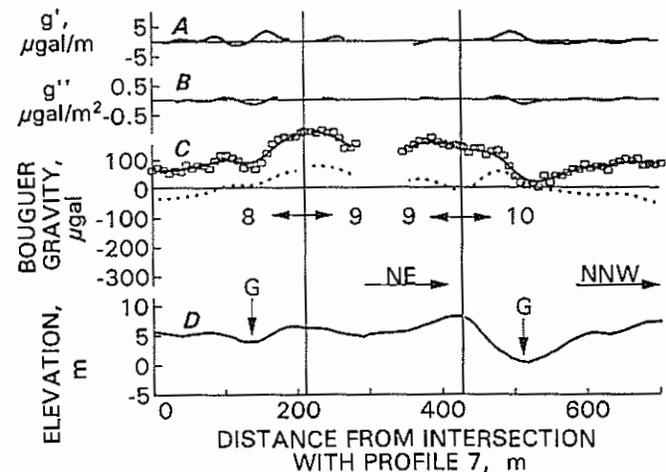
Figure 7. Profiles 8, 9, and 10: A, smoothed first horizontal difference,  $g'$ ; B, smoothed second horizontal difference,  $g''$ ; C, residual Bouguer gravity,  $g$ , (open squares) and smoothed gravity using Bouguer densities of 2.05 (solid curve) and 2.50 (dotted curve) mt/m<sup>3</sup>, respectively; D, elevation above datum. Relative minima of  $g$  (using the lesser Bouguer density) occur in the gully (G) traversed by profiles 8 and 10.
