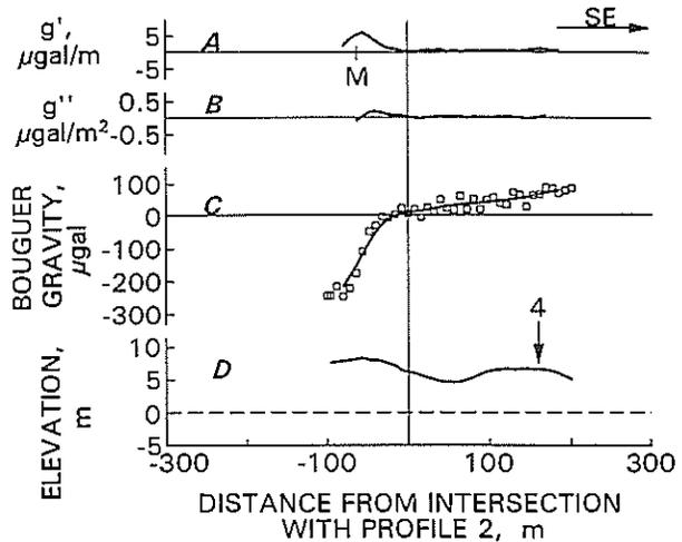
Figure 4. Profile 3: A, smoothed first horizontal difference,  $g'$ ; B, smoothed second horizontal difference,  $g''$ ; C, residual Bouguer gravity (open squares) and smoothed gravity (solid curve); D, elevation above datum. The maximum of  $g'$  occurs above the known mine edge (M). An arrow locates the intersection with profile 4.
