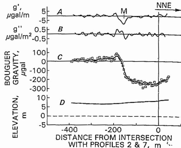
Figure 2. Profile 1: A, smoothed first horizontal difference,  $g'$ ; B, smoothed second horizontal difference,  $g''$ ; C, residual Bouguer gravity,  $g$ , and smoothed gravity (solid curve); D, elevation above datum. The minimum of  $g'$  occurs above the known mine edge (M) located by electromagnetic mapping.
