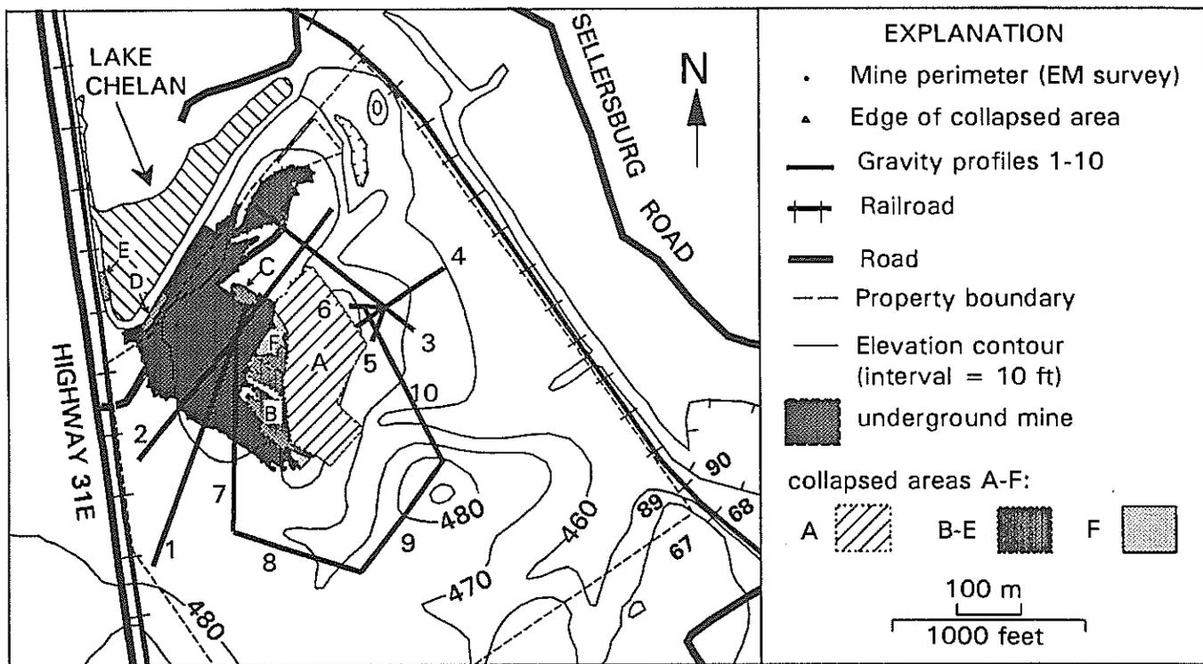
Figure 1. Map of the Falls City Mine showing the uncollapsed portion of the mine as mapped with an underground electromagnetic transmitter and aboveground receiver, collapsed areas, and gravity profiles 1-10. The indicated property boundary includes the southeast and northeast boundaries of Clark Military Grant 89. Collapsed areas were mapped with the aid of aerial photographs.
