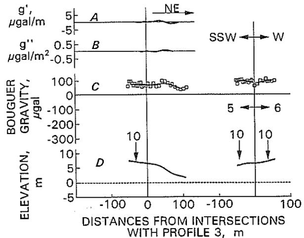
Figure 5. Profiles 4, 5, and 6: A, smoothed first horizontal difference,  $g'$ ; B, smoothed second horizontal difference,  $g''$ ; C, residual Bouguer gravity (open squares) and smoothed gravity (solid curve); D, elevation above datum. Arrows locate intersections with profile 10.
