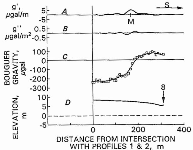
Figure 6. Profile 7: A, smoothed first horizontal difference,  $g'$ ; B, smoothed second horizontal difference,  $g''$ ; C, residual Bouguer gravity (open squares) and smoothed gravity (solid curve); D, elevation above datum. The maximum of  $g'$  occurs above the known mine edge (M). Profile 8 starts at the southern end of profile 7.
