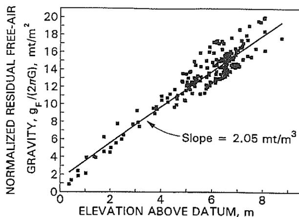
Figure 8. Normalized residual free-air gravity,  $g_f/2\pi G$ , in profiles 1-10 versus elevation above datum. The plotted straight line, obtained by linear regression, has a slope of  $2.05 \text{ mt/m}^3$ . The data are from all off-mine stations more than 20 m from collapsed areas and more than 50 m, along the direction of profile, from the uncollapsed mine perimeter.
