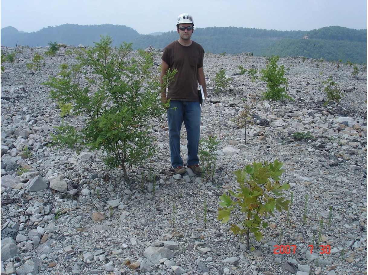
Figure 3. Gray sandstone plot after three growing season at Catenary Coal Mine, Kanawha County, West Virginia.
