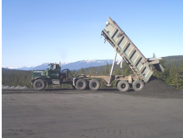
Figure 3. 40-tonne haul truck dumping a load of tailings.
