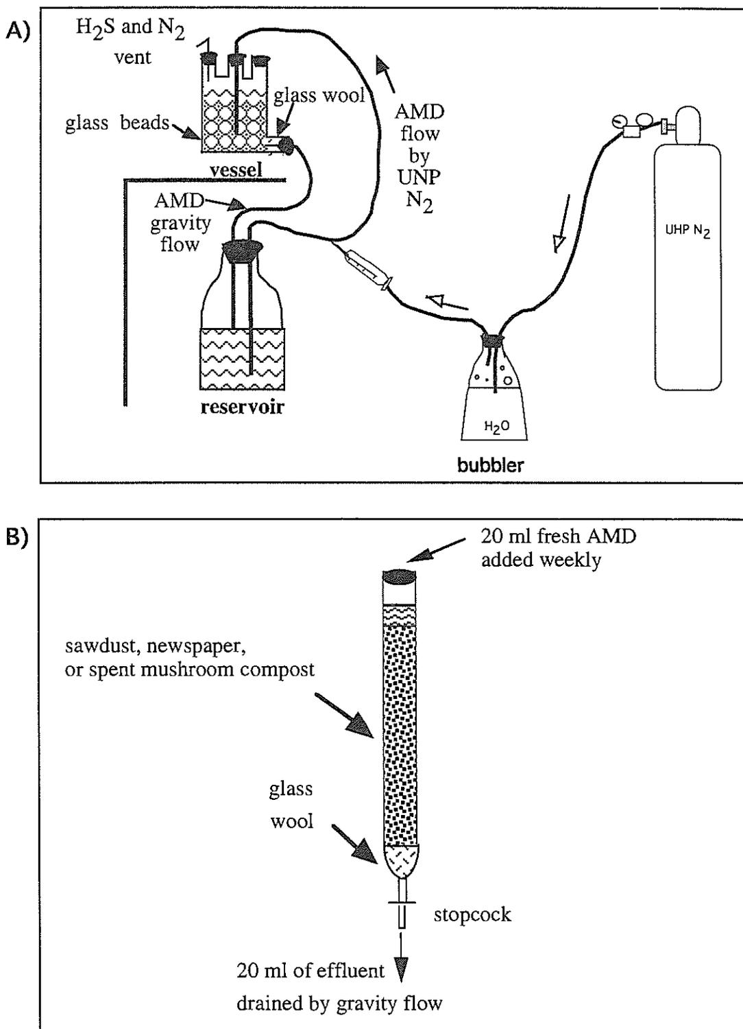
Figure 2. A) Reaction vessel and reservoir . B) Column design. Weekly, 20 ml of effluent was drained from the stopcock and fresh AMD was replaced at the top.
