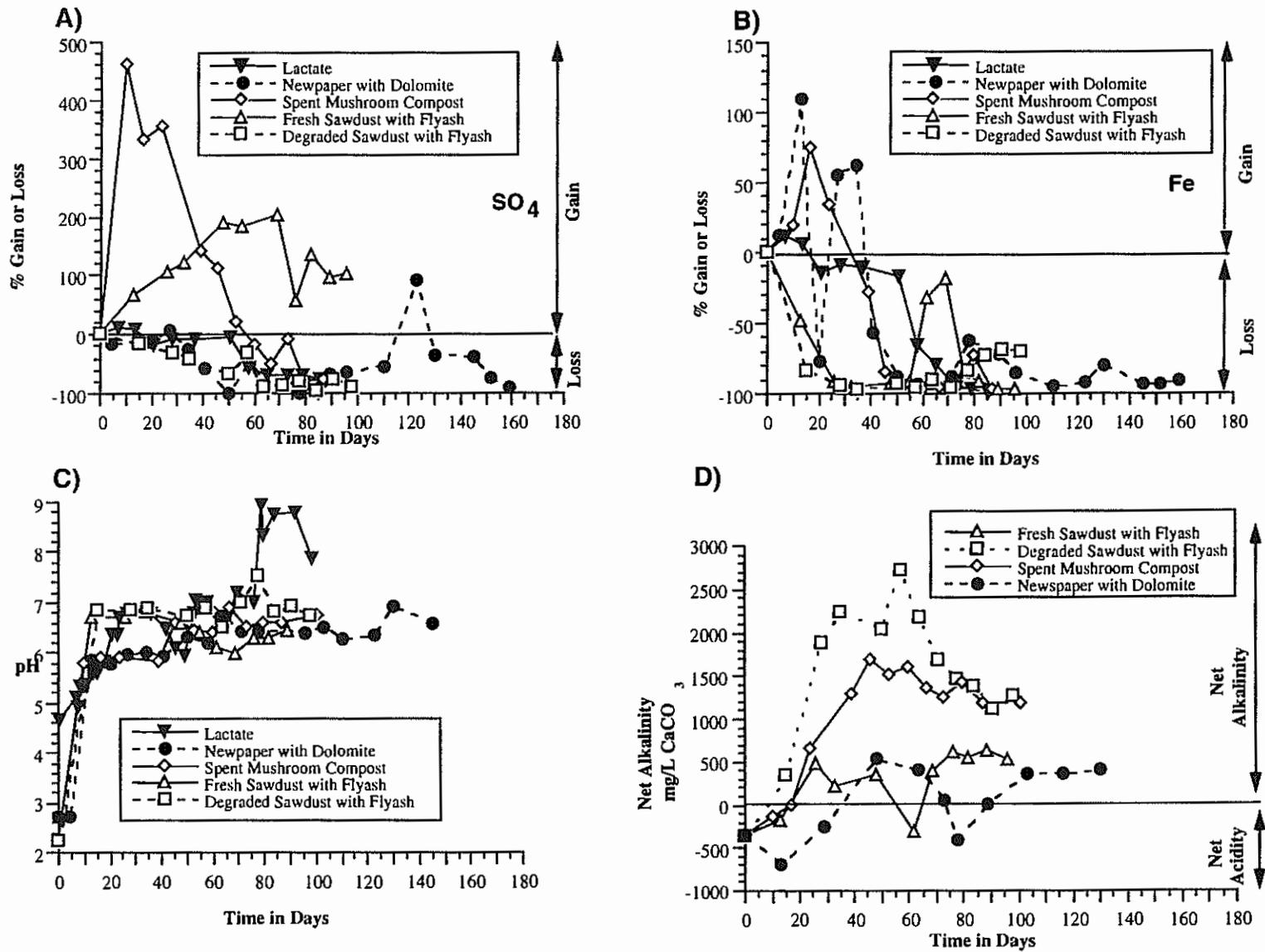
Figure 4. Experimental data for various organic substrates tested in the lab. A) and B) Gains and losses for sulfate and iron are expressed in % relative to the influent concentrations; C) pH over time; D) Net alkalinity over time.
