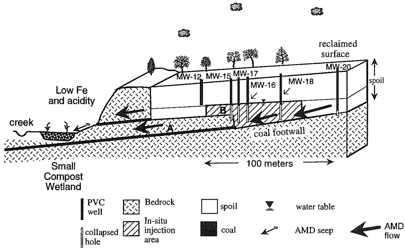
Figure 1. Schematic diagram of the area of in-situ sulfate reduction. Wells at the site are indicated. A hypothetical wetland is included in the diagram. Thick arrows indicate possible ground water flow paths. A) AMD may flow between the Mercer and Brookville coals in a sandstone unit and emerge as seeps along the crop line. B) This may be an area of little flow. Due to the shallow water table in this area, anaerobic conditions may not be maintained here.
