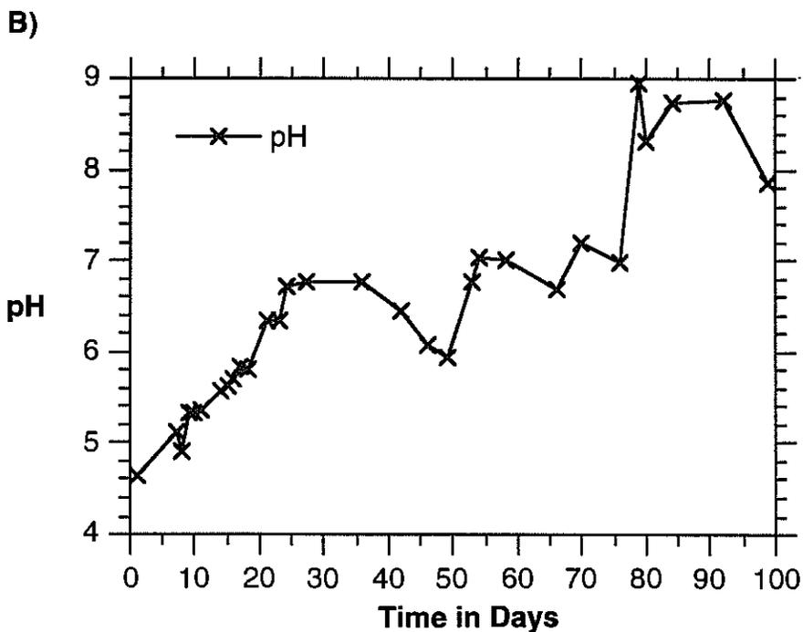
Figure 3. Plot of sulfate, iron (A) and pH trends (B) over time for the lactate experiment as an example of the raw data. The lag time before sulfate reduction is between day 0 and day 15. Sulfate decreases rapidly after this period. The ceasing of sulfate reduction from day 30 to day 55 represents a period of negligible organic matter concentrations. Sulfate decreases again when lactate is added on day 46.
