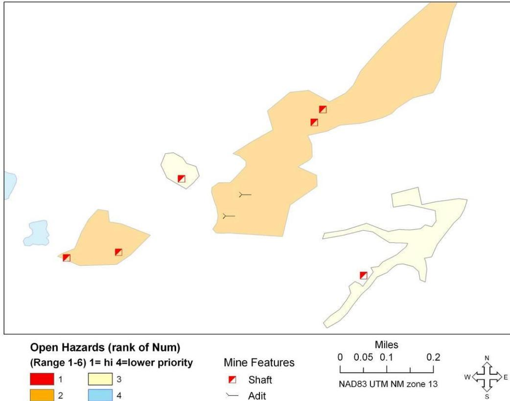
Figure 7. Method used to calculate open hazard priority. The rank of open hazards range between 1 and 6. Natural breaks in the data were used to classify these values into 4 priority groups.
