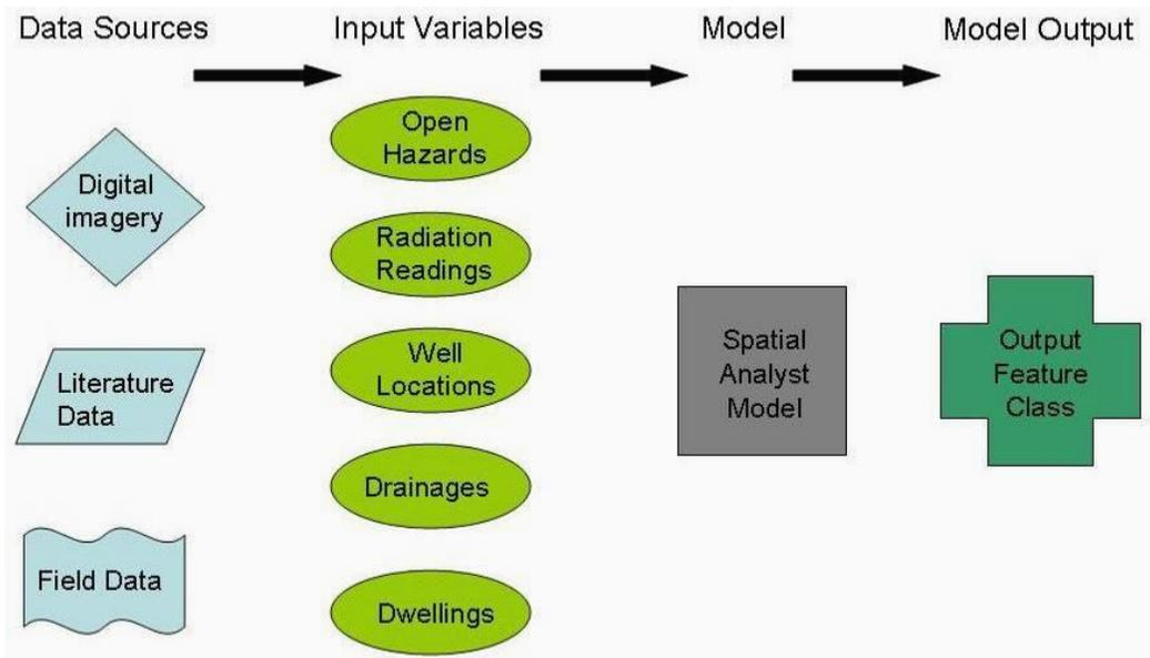
Figure 6: Abandoned uranium mine prioritization model schematic.
