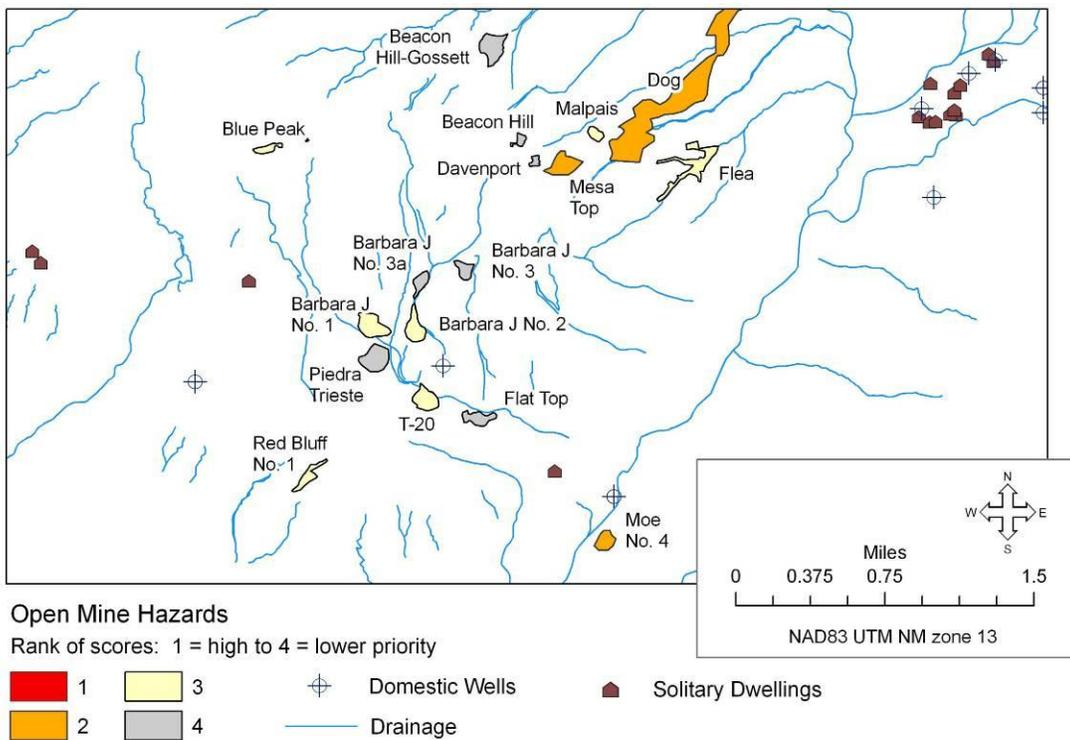
Figure 14. Priority ranking of abandoned uranium mines in the San Mateo Creek watershed based on the number of open hazards.
