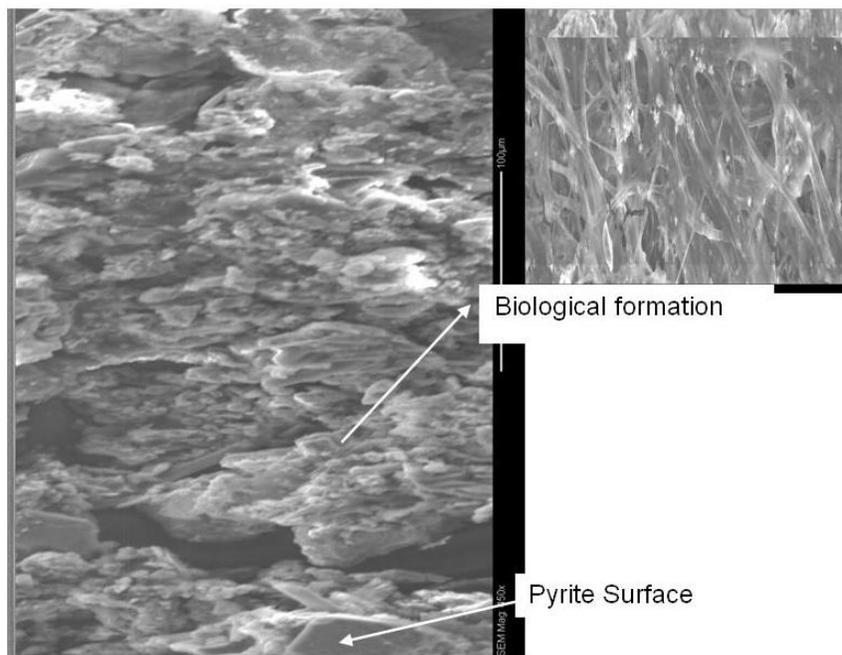
Figure 7. Biochemical Film Structure on AMD Source.
