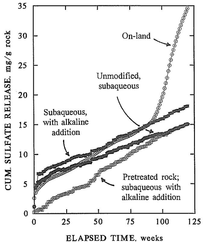
Figure 3. Cumulative sulfate release for on-land and subaqueous disposal. The rates of sulfate release and attendant acid production for the disposal options did not differ greatly. Data presented are from the second replicates.
