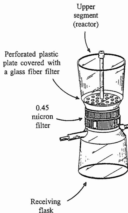
Figure 1. Reactor design.
