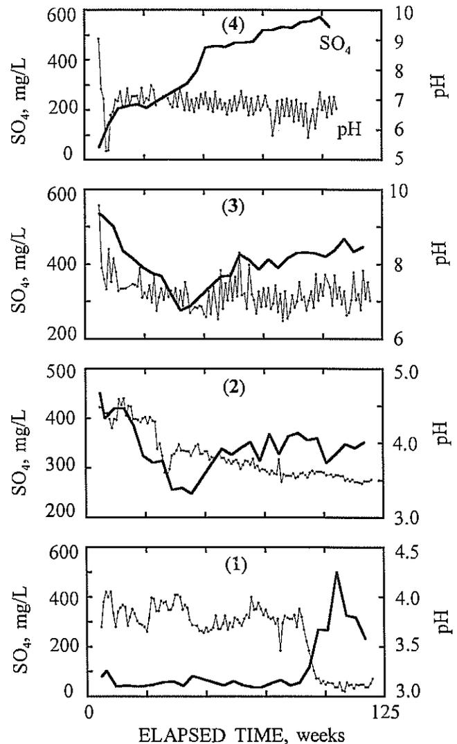
Figure 2. Solution pH and sulfate concentrations for (1) on-land disposal, (2) unmodified subaqueous disposal, (3) subaqueous with alkaline addition, (4) pretreated rock, subaqueous disposal with alkaline addition. Acidic solutions were produced by (1) and (2).
