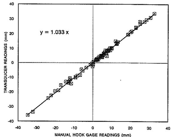
Figure 7. Plot of 84 daily transducer readings vs. hook gage readings.
