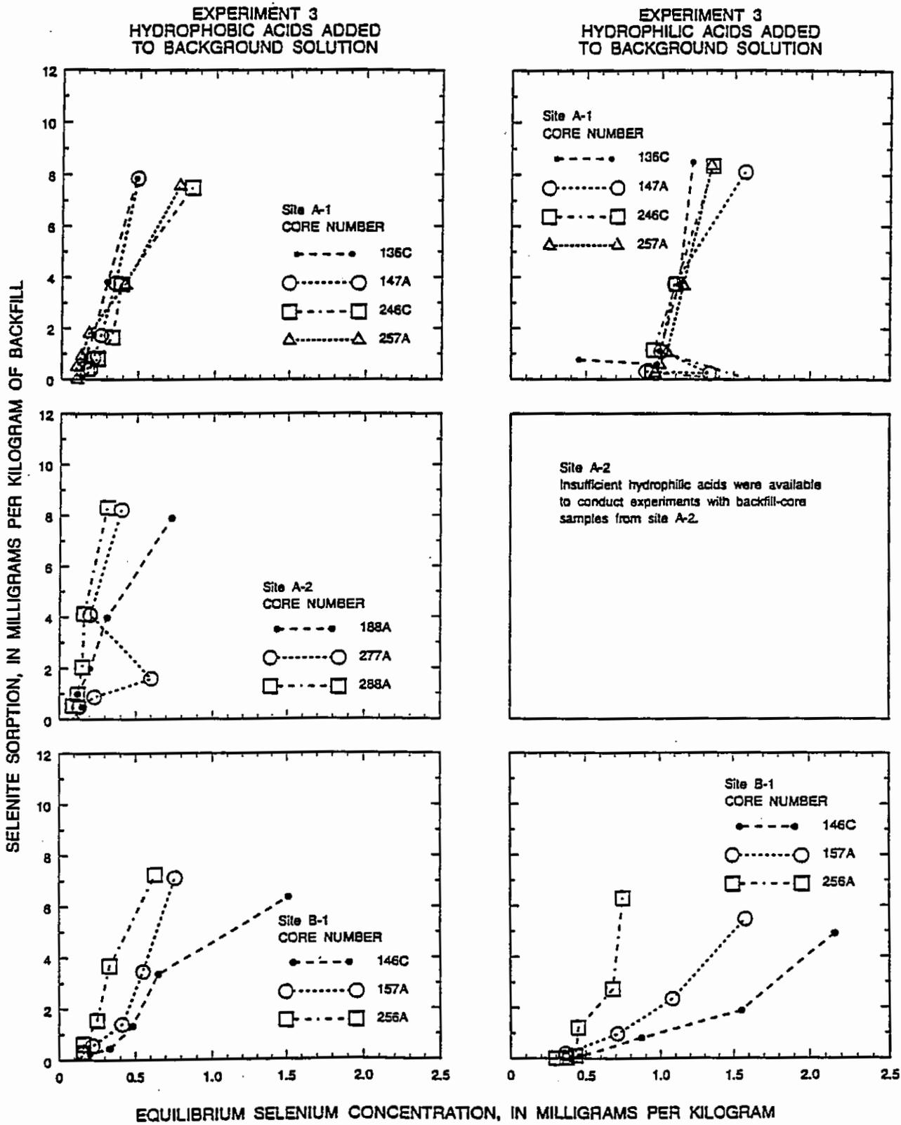
Figure 3. Selenite sorption as a function of equilibrium selenium concentrations of backfill-core sample solutions with hydrophobic and hydrophilic acids added to background solutions.
