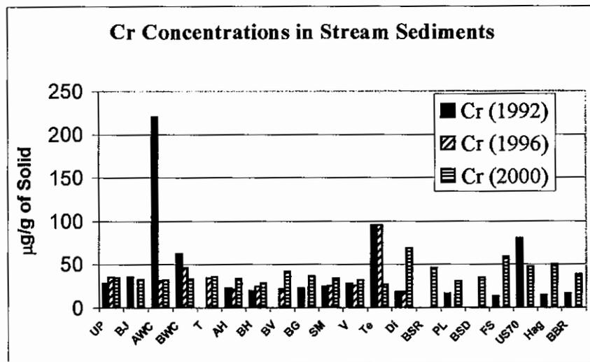
FIGURE 7. Comparison of chromium concentrations in stream sediments.
