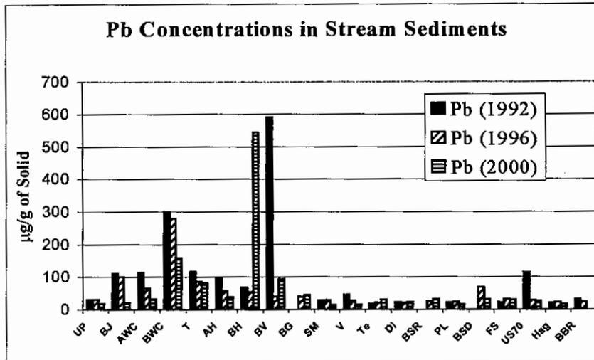
FIGURE 6. Comparison of lead concentrations in stream sediments.
