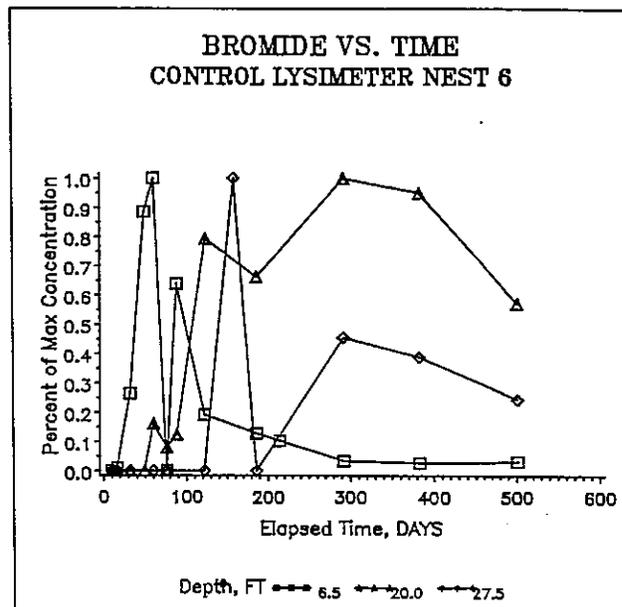
Figure 7. An example plot of normalized Br concentrations versus time. Background concentration is below detection limits (20 ppb). Application date is day zero.
