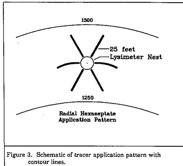
Figure 3. Schematic of tracer application pattern with contour lines.
