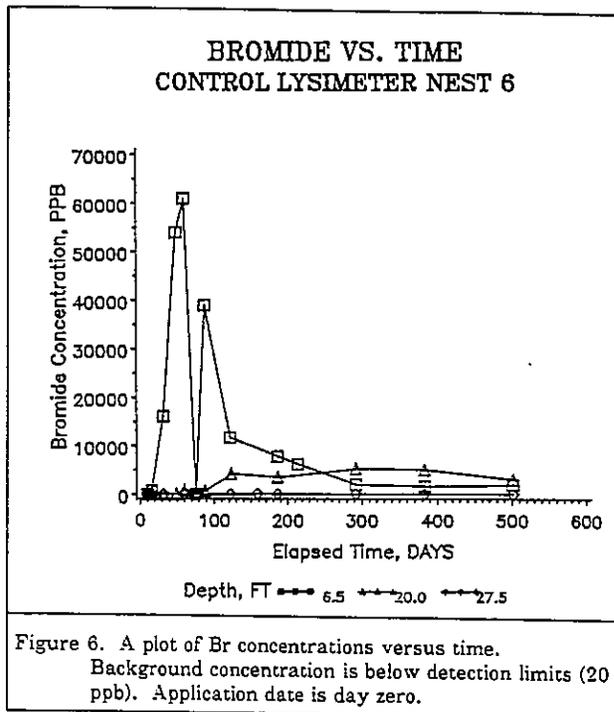
Figure 6. A plot of Br concentrations versus time. Background concentration is below detection limits (20 ppb). Application date is day zero.
