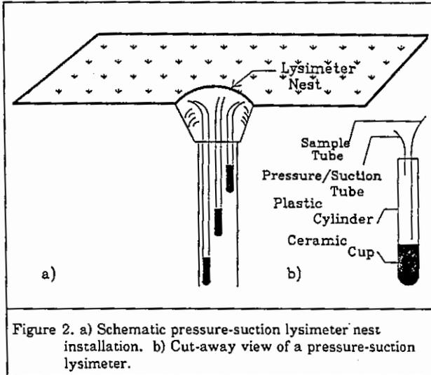
Figure 2. a) Schematic pressure-suction lysimeter nest installation. b) Cut-away view of a pressure-suction lysimeter.
