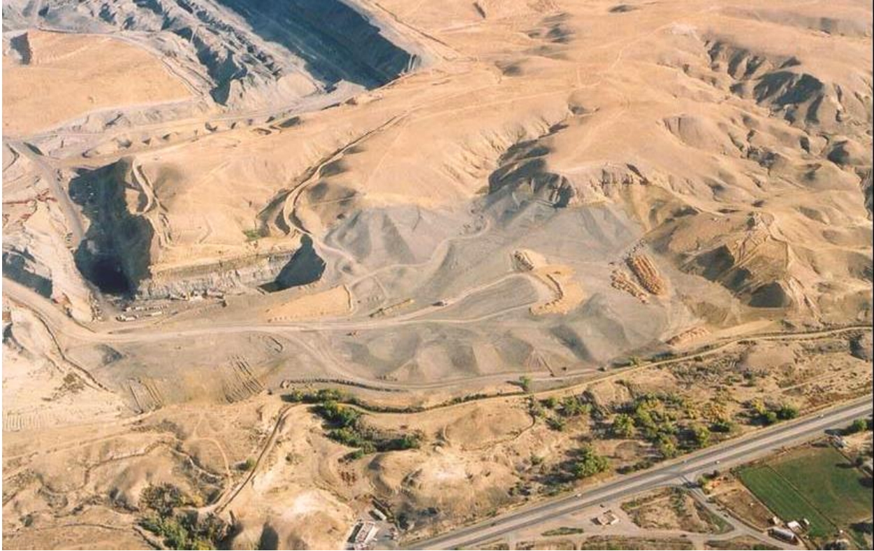
Figure 7. Fluvial geomorphic reclamation is underway at the 115-acre Cottonwood Reclamation Project, Farmington, New Mexico.
