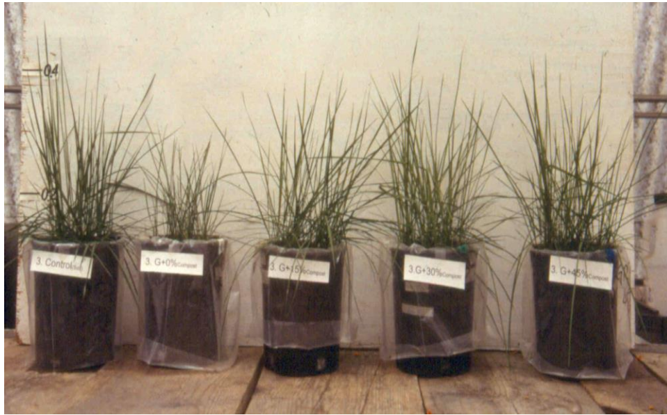
Figure 3. Tall fescue response to additions of papermill sludge compost to hard rock mine residuals. Treatments from left to right are prime farmland control topsoil (Orangeburg series) and 0, 15, 30, and 45% compost by volume added to mixture of mineral fines and crushed overburden. In general, results from this trial and others have led to a base recommendation of 15 to 20% compost by volume in manufactured soil mixes such as these.
