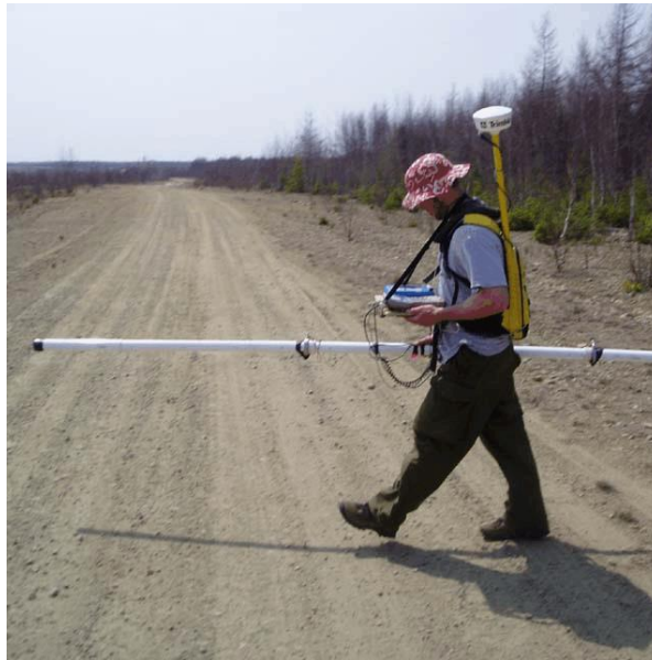
Figure 3. Student carrying the EM31, the backpack-mounted DGPS and their respective data loggers during UNB field school in May 2004.
