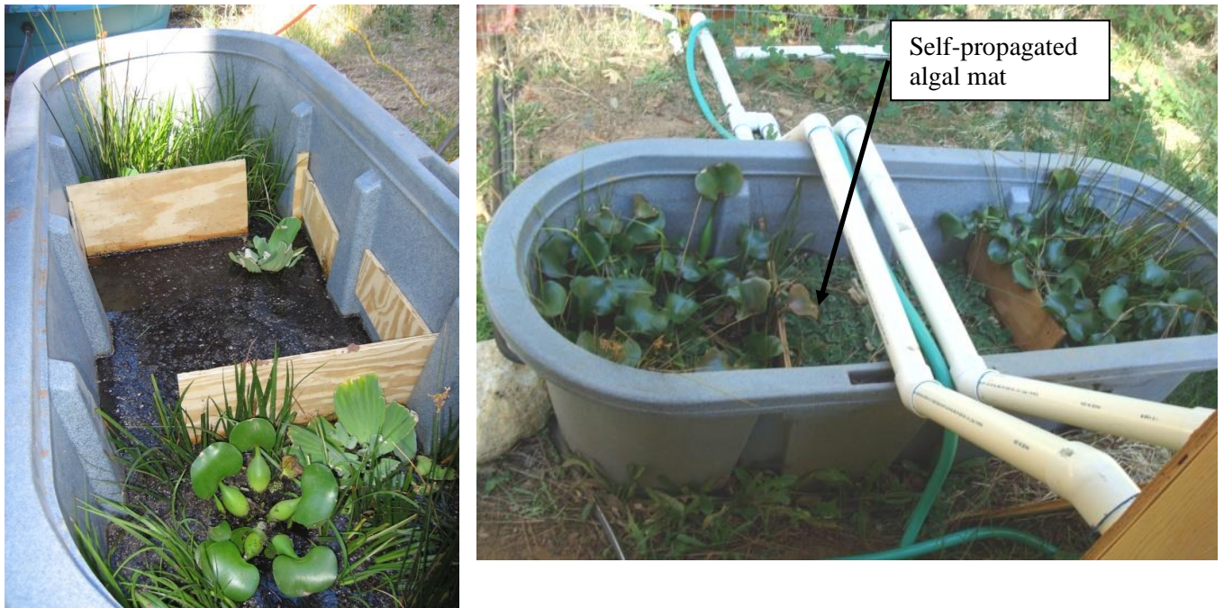
Figure 3. Initial (left) and 10-week-old (right) bench test wetland cells
