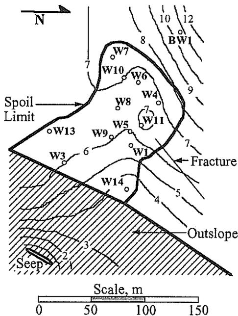
Figure 3. Water table contours (m) at steady-state (low-flow) conditions, August 29, 1990.
