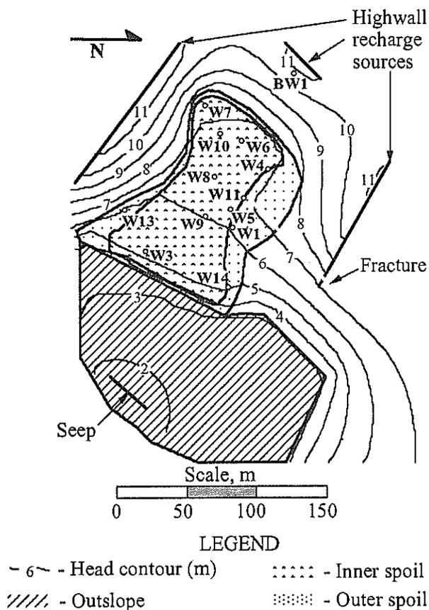
Figure 5. Head contours generated from MINEFLO model, 1990 simulation.
