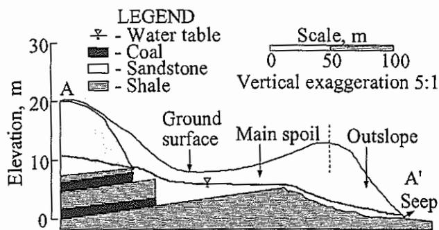
Figure 2. Cross-section of mine spoil study site.
