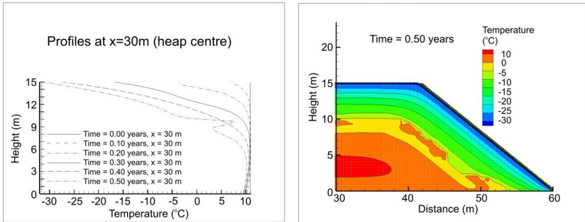
Figure 4. Simulated waste rock pile temperatures in the first six months, based on an oxidation rate of  $10^{-9}\text{ kg } (\text{O}_2)\text{ m}^{-3}\text{ s}^{-1}$ .
