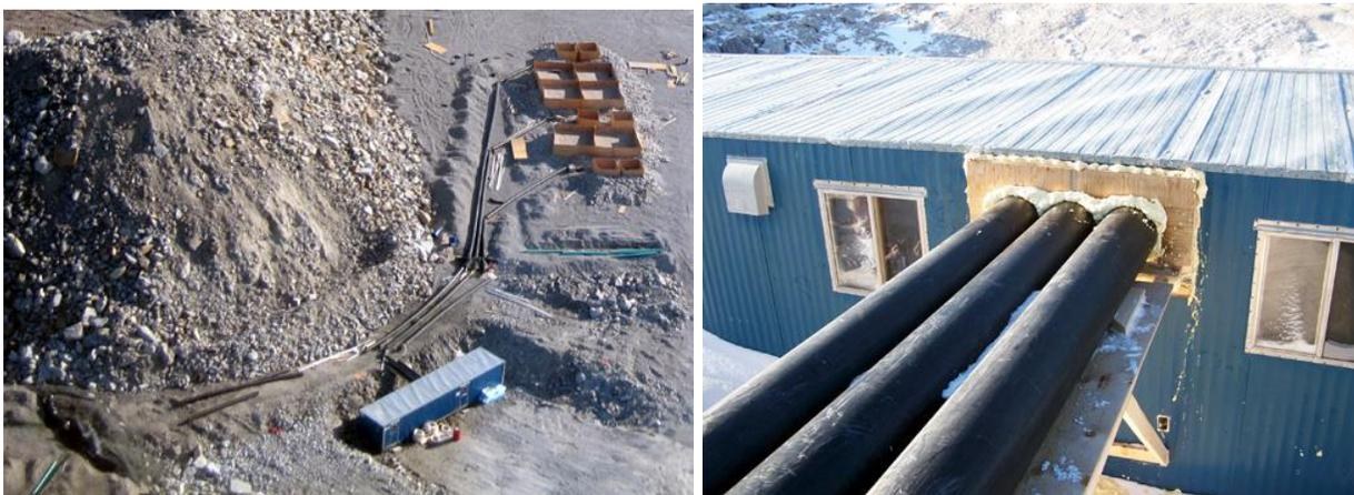
Figure 9. Photo to the left shows cluster lysimeter drainage pipes directed into the instrumentation shack. The instrumentation shack is situated between the Type I and Type III rock pads. The photo to the right shows lysimeter drainage pipes entering the instrumentation shack.
