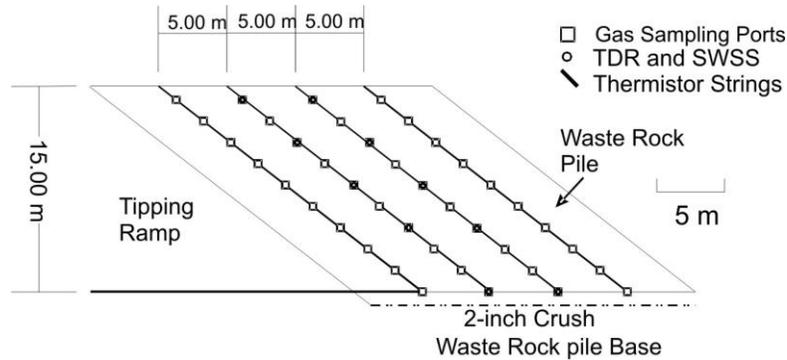
Figure 11. Cross-section of a waste rock pile showing the instrumentation along the tip faces (TDR = time domain reflectance probes and SWSS = soil water suction sampler).
