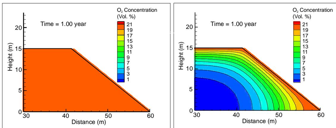
Figure 5. Simulated distribution of oxygen in the heap (1 year) for two different oxidation rates,  $10^{-9}$  and  $10^{-8}$   $\text{kg}(\text{O}_2) \text{m}^{-3}\text{s}^{-1}$ , respectively.
