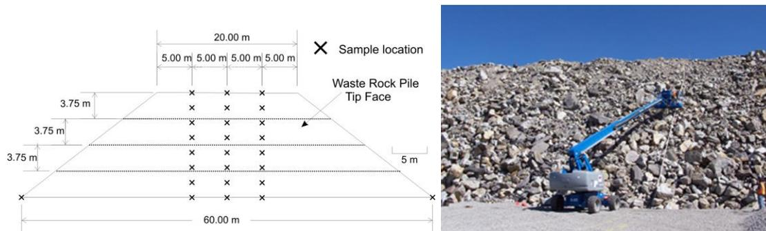
Figure 2. Diagram to the left is a cross-section of a waste rock pile showing waste rock sampling locations along the tip face. Three to four tip faces will be sampled for each pile. The photo to the right shows the sampling procedure on the tip face.
