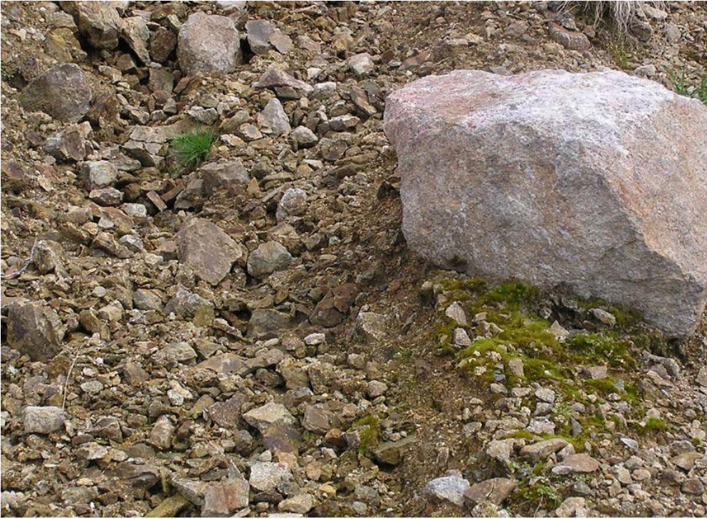
Figure 3. Moss cover on the granite pit wall 12 months after application in the hydroseeding mixture trial, on a plot that was treated with a mixture containing high soil additive levels. The footprint (bottom left) shows the fragile nature of this surface. Note the untreated slope behind with no vegetation.
