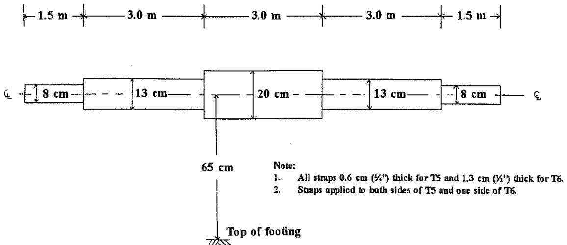
FIGURE 4 STEEL REINFORCING STRAP DIMENSIONS FOR WALLS T5 AND T6
