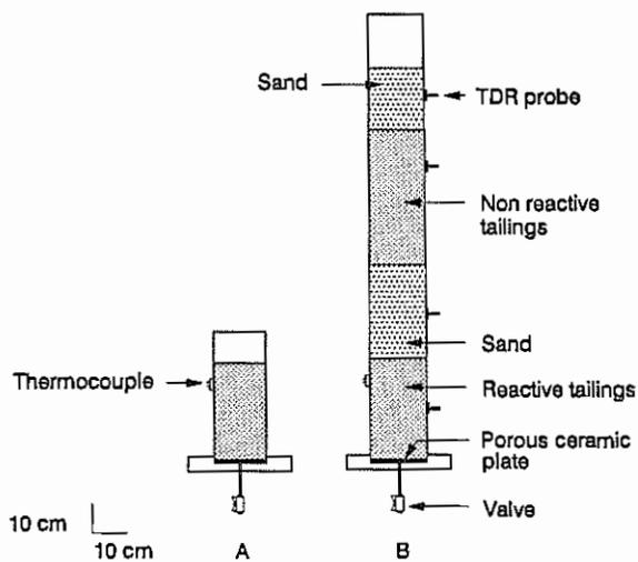
Figure 3. Schematic representation of the control columns;
