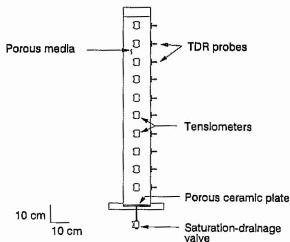
Figure 2. Schematic representation of the drainage column.
