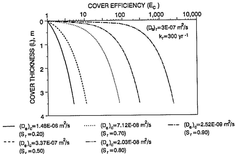
Figure 5. Relationship between the cover thickness and its efficiency to reduce the oxygen flux (after Achib et al. 1993).
