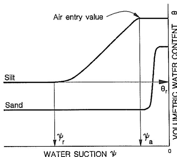
Figure 1. Typical moisture characteristic curves.
