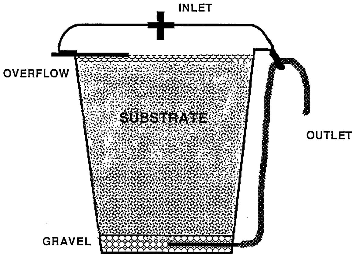
Figure 1. Typical bench scale wetland module in downflow configuration.
