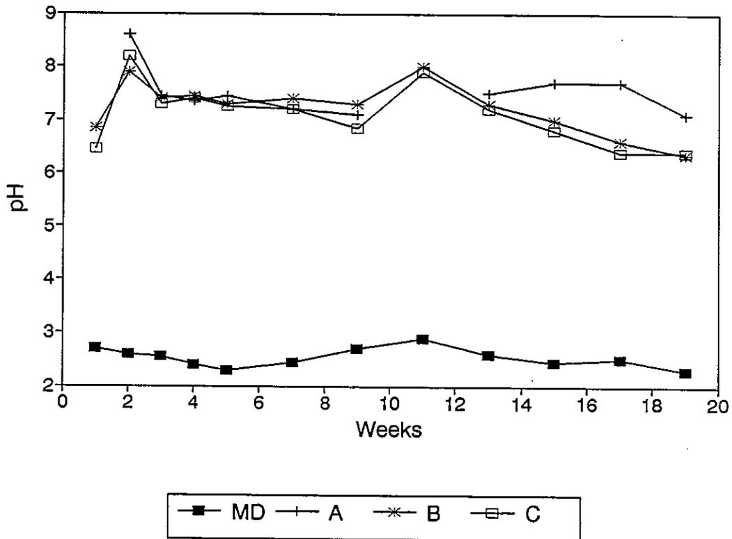
Figure 2. pH of mine drainage and permeameter effluents for National Tunnel and Quartz Hill Tunnel.
