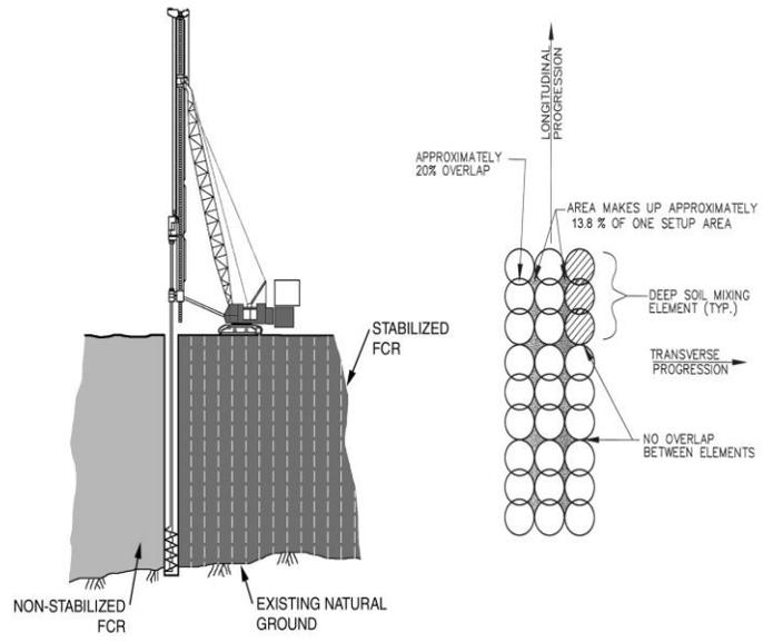
Figure 6. Deep soil mixing procedure.
