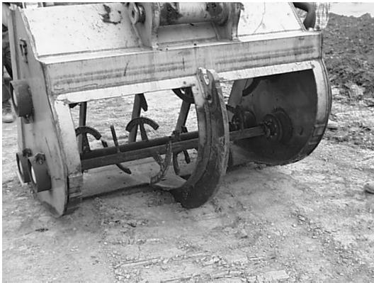
Figure 3. Shallow soil mixing bucket.
