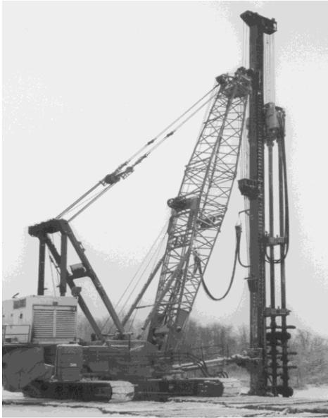
Figure 5. Deep soil mixing augers.
