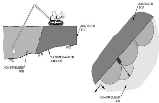
Figure 4. Shallow soil mixing.
