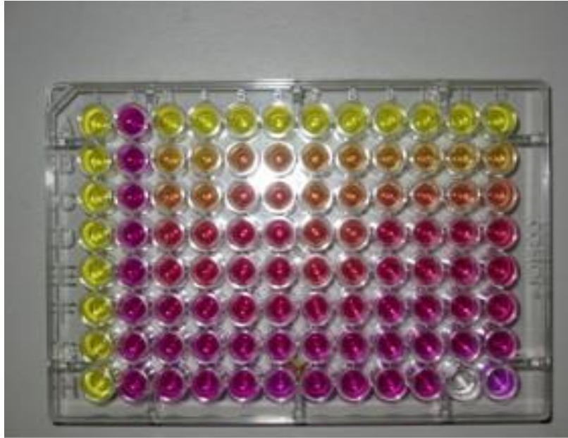
Figure 2 - MetPLATE™ 96-well Microplate with Colorometric Response
