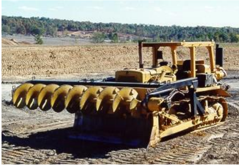
Figure 1. Mechanical system for reconstructing soil mounted on a conventional bulldozer, before improvements.
