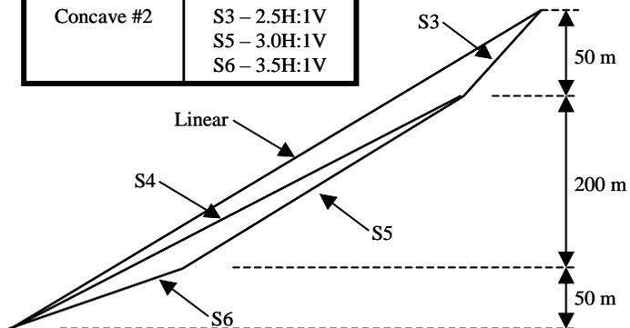
Figure 4. Slope profile designs examined in the erosion modeling program for the small and large waste rock stockpile at the case study #1 site.
