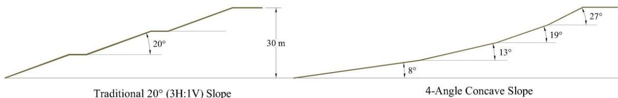
Figure 3. Schematic showing traditional and concave slope designs for reclaimed waste rock stockpiles.
