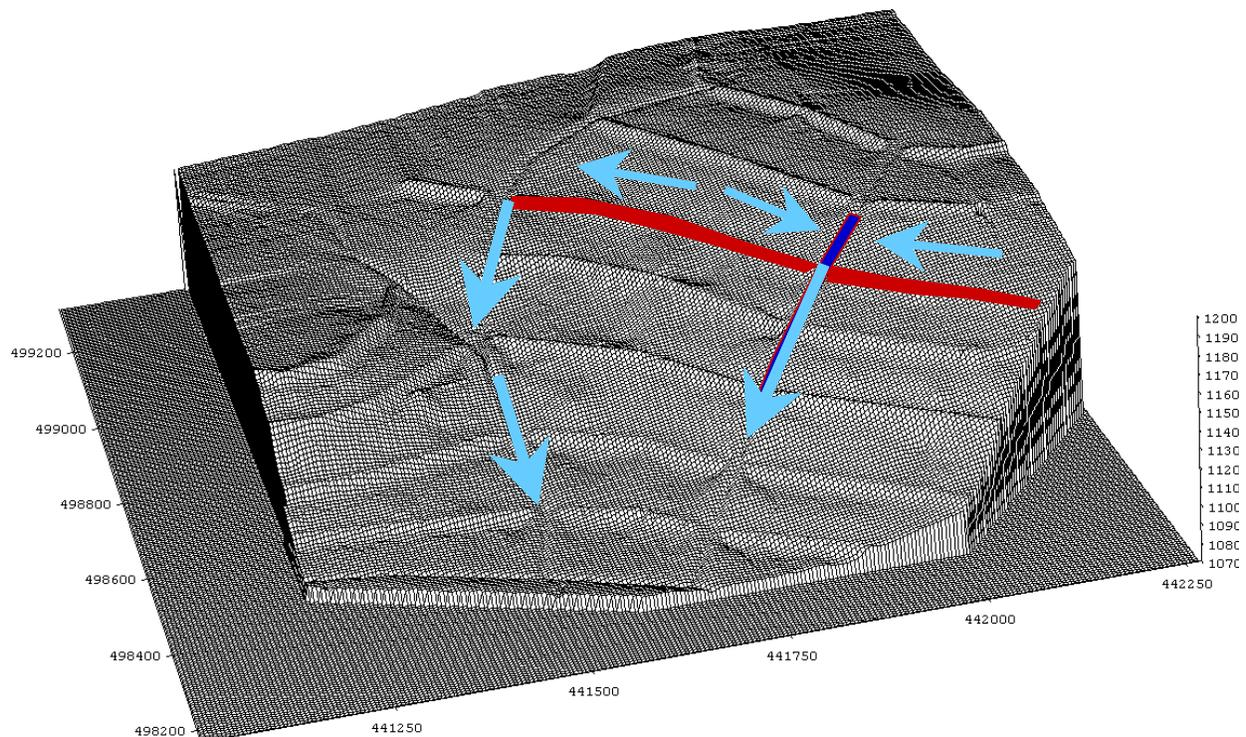
Figure 6. Surface contours (vertically enhanced) for the first landform alternative evaluated for the Whistle Mine backfilled pit cover system (from Ayres et al., 2005).
