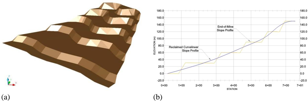
Figure 9. (a) Perspective view and (b) slope profiles for a contour-terraced waste rock stockpile.
