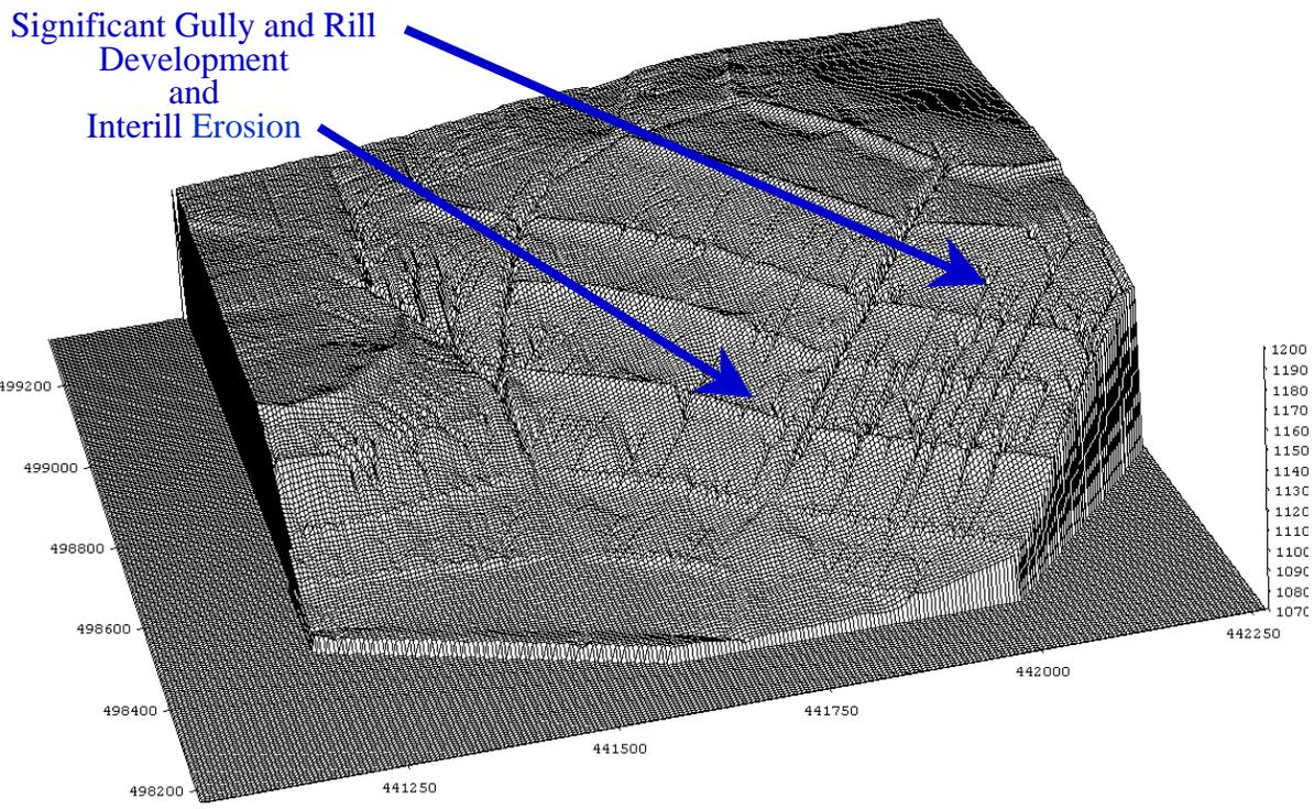
Figure 7. Predicted landform evolution of the first landform alternative for the Whistle Mine backfilled pit cover system after 100 years (from Ayres et al., 2005).
