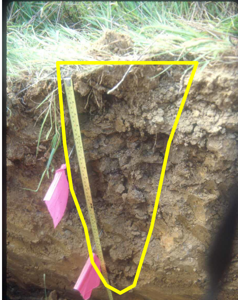
Fig. 12. The effect of ripping on the soil structure five years after the treatment was performed.
