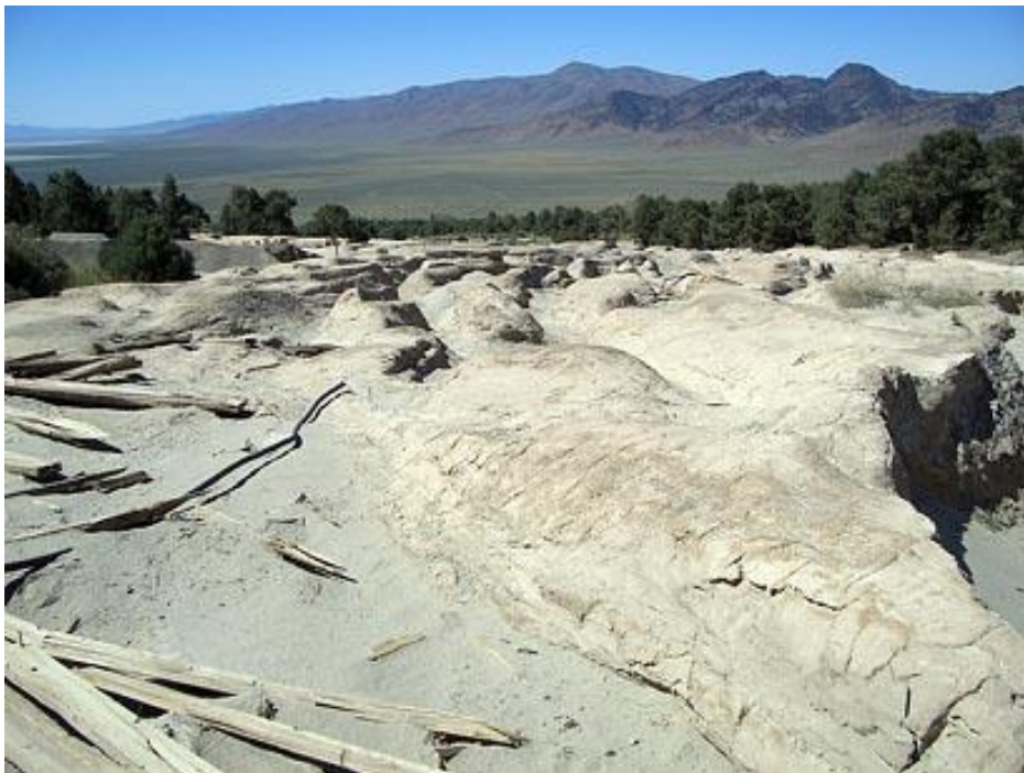
Figure 1. Early 20th Century tailings disposal at an abandoned gold mine in Nevada, USA (Martin et al, 2002)
