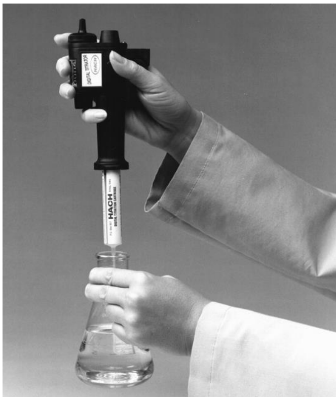
Figure 2. Measuring Alkalinity using a digital titrator.
