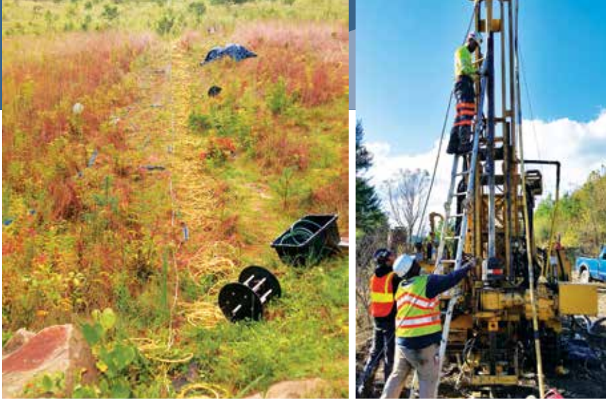
Figure 2. ERI and artificial rainfall (sprinklers) at Barton Hollow fill (left), and drilling at Office Fill (right). (Photo credits to Kathryn Little (left), and Joseph Buckwalter (right)).
