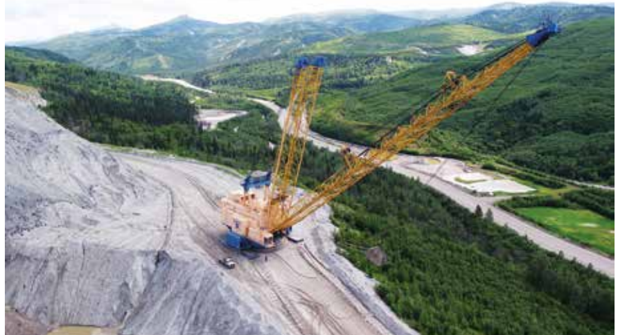
Figure 2. Bucyrus-Erie 1300W dragline, named "Ace in the Hole," moves the overburden overlying the coal seams at Poker Flats and Two Bull Ridge Mines.
