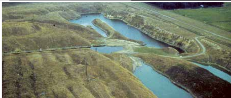
Figure 3. Surface mining before passage of reclamation laws in Illinois often resulted in abandoned highwalls, pits of water, and undulating land surface due to ungraded, weathered spoil ridges.
