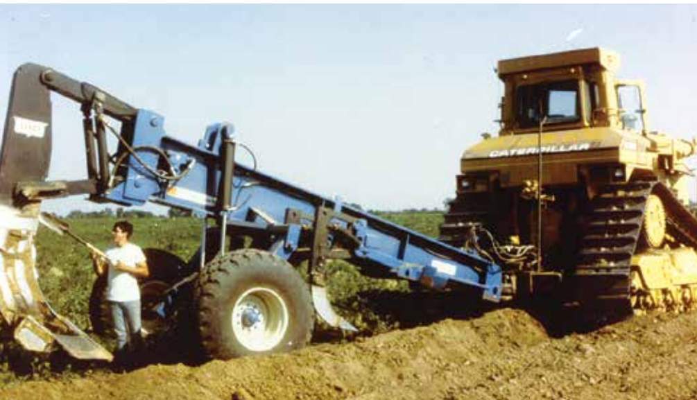
Figure 4. Deep tillage equipment to reduce soil compaction on Illinois surface mines after 4 feet of topsoil was replaced.
