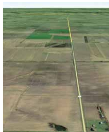
Figure 9. Aerial view of the same area in Figure 8 after reclamation had filled subsidence depressions and restored drainage patterns.
