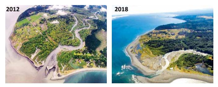
Figure 3. As the dams were being decommissioned, there was an influx of sedimentation flowing from the Elwha River. It is estimated that 4 million metric tons of sediment accumulated in the river delta. This resulted in depositing a meter of sedimentation in the estuary, expanding the beach 400 m, and creating new landforms at the river's mouth. Photo credit: Tom Roorda.
